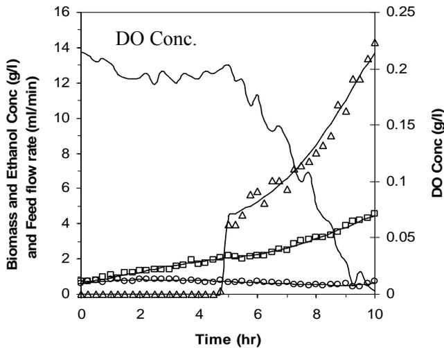
Fig. 6 Implementation of Control Strategy I simulated ( — from model,  $\circ$  Ethanol Conc.,  $\square$  Biomass Conc.,  $\Delta$  Feed flow rate)
