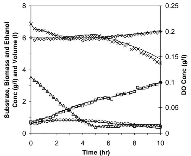
**Fig. 5** Generalization profiles of SAN for training data set simulated ( — from model,  $\circ$  Ethanol Conc.,  $\square$  Biomass Conc.,  $\Delta$  Substrate Conc.,  $\diamond$  Volume of reactor and  $\times$  DO Conc.)
