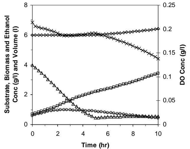
**Fig. 4** Recall profiles of SAN for training data set simulated ( — from model,  $\circ$  Ethanol Conc.,  $\square$  Biomass Conc.,  $\Delta$  Substrate Conc.,  $\diamond$  Volume of reactor and  $\times$  DO Conc.)
