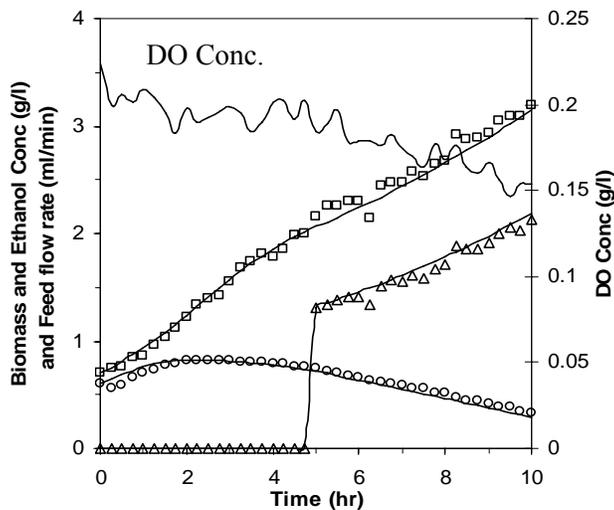
Fig. 7 Implementation of Control Strategy II simulated ( — from model,  $\circ$  Ethanol Conc.,  $\square$  Biomass Conc.,  $\Delta$  Feed flow rate)
