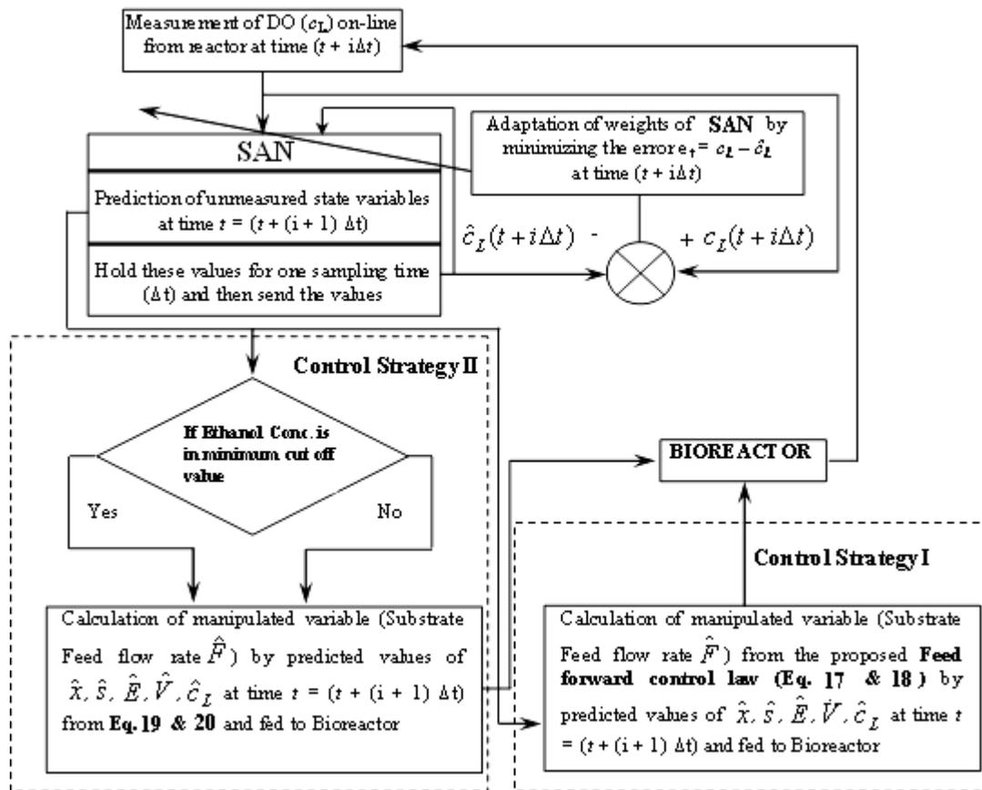
Fig. 2 Flow diagram of SAN application in control strategies for Fed-batch fermentation
