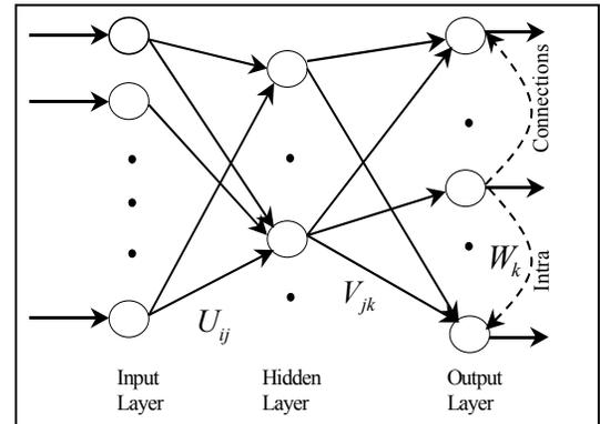
Fig.1b Schematic diagram of feed-forward neural network for each sub-network of SAN
