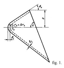
The control of such vehicle is carried out by change of its roll angle on constant zero balance of attack angle. It allows to consider the flow process around nose part of the vehicle as axisymmetrical. The exact account of mass ablation, even for so easy configuration at above simplifying assumptions is difficult. Therefore we shall enter some more assumptions for the vehicle of this form:
