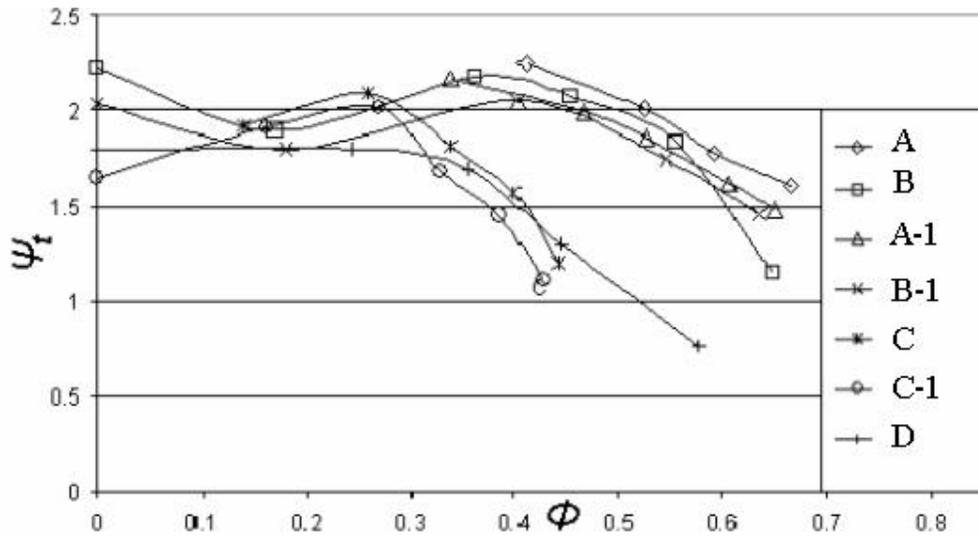
Fig. 2: Grouping of squirrel cage fan performance curves according to volute size using common definitions of head and flow rate coefficients.
