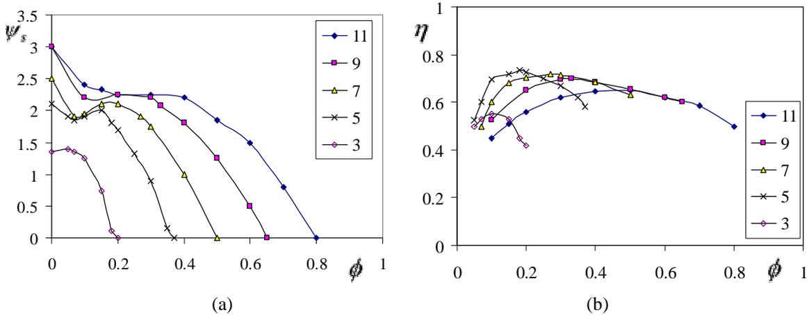
Fig. 4: Fan performance curves for different volute spread angles (degrees) using common definition of the flow coefficient. [7]. a): static head coefficient. b): efficiency.
