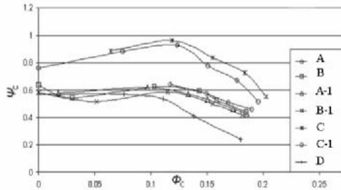
Fig. 3: Grouping of squirrel cage fan performance curves according to volute size using casing based non dimensional coefficients
