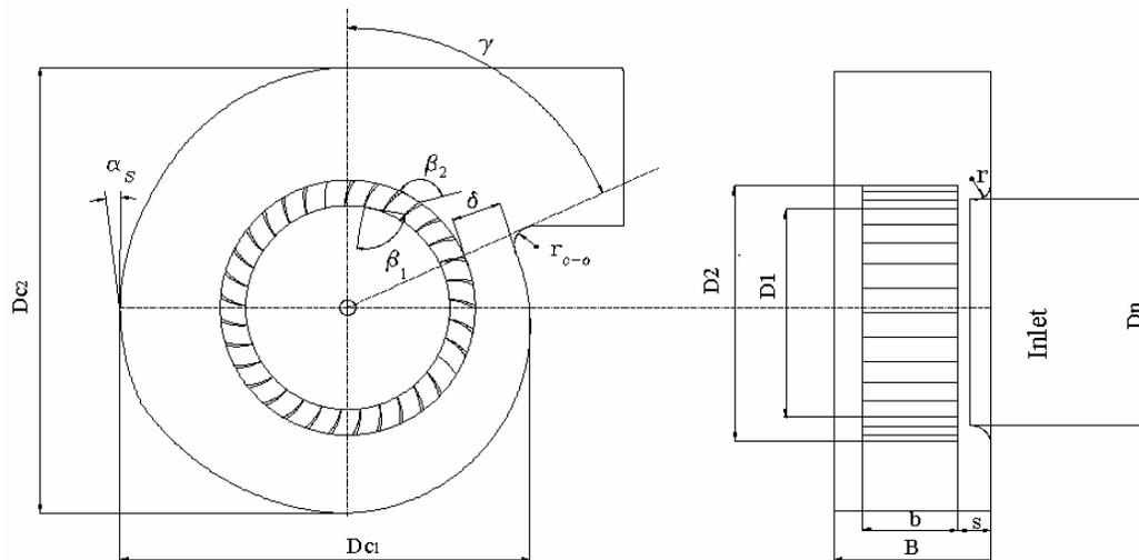
Fig. 1 A general schematic and geometries of squirrel-cage fan
