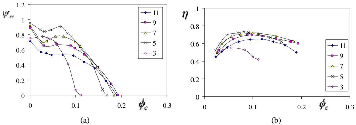
Fig. 5: A comparison between squirrel cage fan performance curves using casing based non dimensional coefficients. a) static head. b) efficiency.
