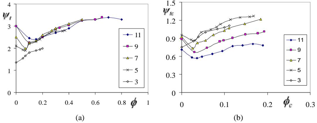
Fig. 6 The advantage of the new definition of non dimensional head in showing an optimum for the volute spread angle. a) rotor based total head coefficient [7]. b) casing based total head coefficient.
