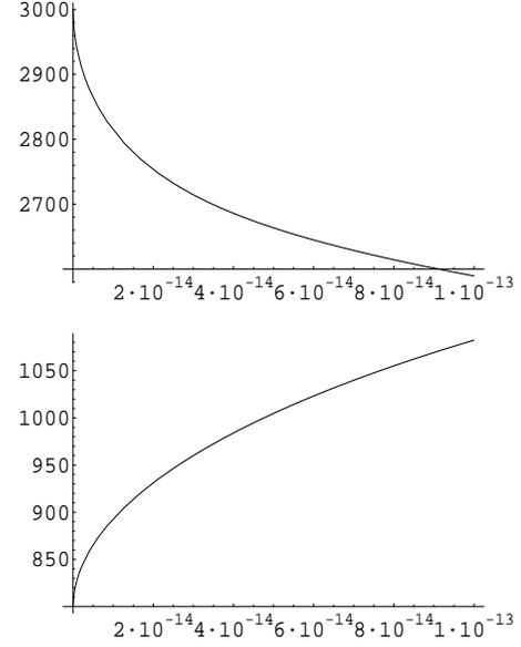
Figure 2: Hyperbolic interface temperature in body 1 (up) and 2 (down).
