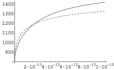
Figure 3: Parabolic (continuous) and hyperbolic (dashed) interface temperature of body 2.
