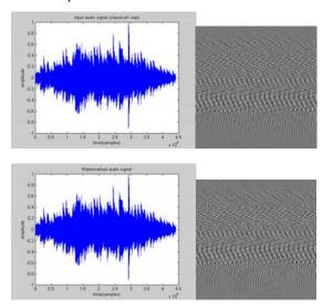
Figure 1. Clockwise: Input original audio signal A; Image  $I_A$ ; Watermarked  $I_A^W$  with PSNR=42.3333 between  $I_A$  and  $I_A^W$ ; Watermarked audio signal  $A_W$ with SNR=32.8782 between A and  $A_W$ .
