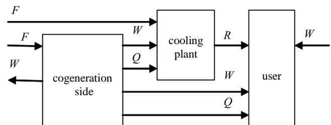
Fig. 1. General CHCP Plant Layout and Energy Flows
