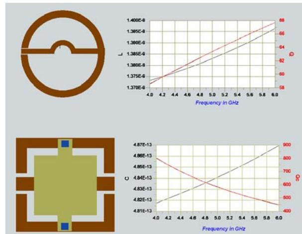
Figure 2. Layout and Q of Passives
