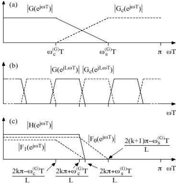
Figure 5: Frequency Response Masking (Case 1)
