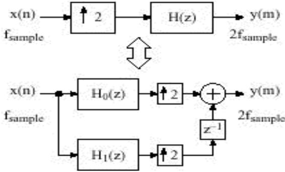
Figure 1: Polyphase interpolator structure
