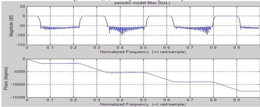
Figure 10: Periodic model filter  $G(z^L)$
