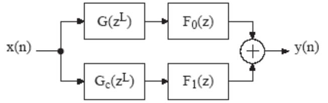
Figure 7: Structure used in the FRM approach
