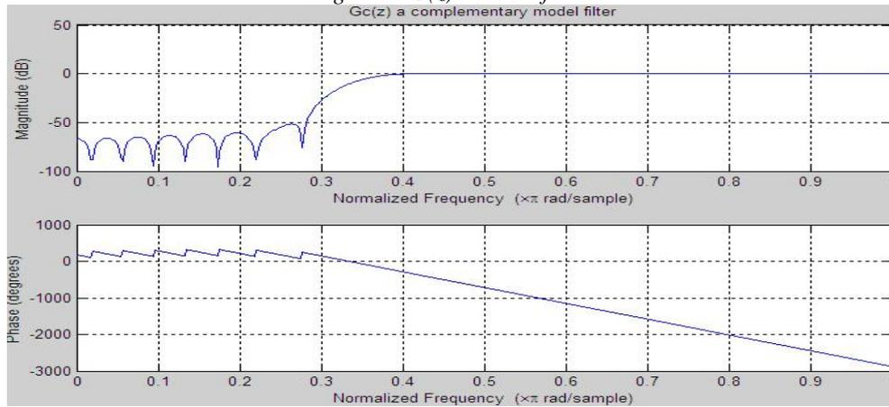
Figure 9:  $G_c(z)$  a complementary model filter
