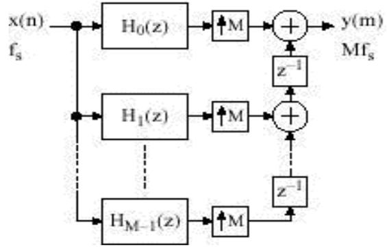
Figure 3 : Polyphase interpolator structure
