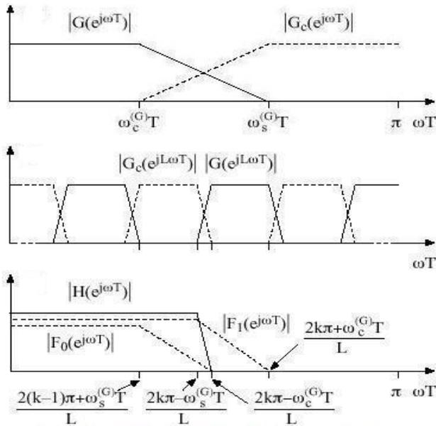
Figure 6: Frequency Response Masking (Case 2)
