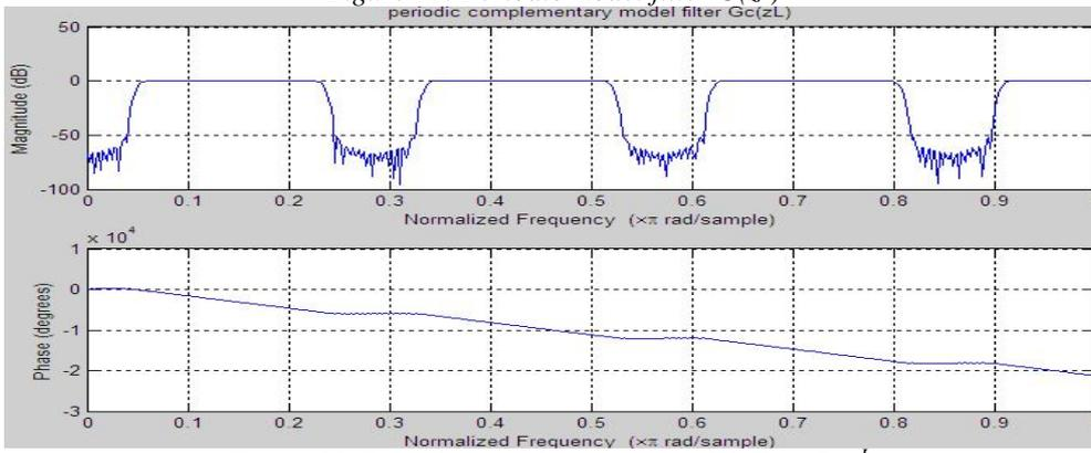
Figure 11: Periodic complementary model filter  $G_c(z^L)$
