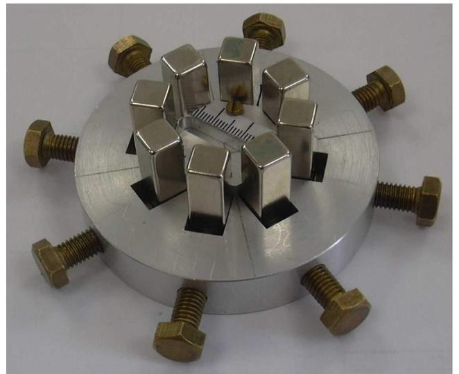
Fig 4: Permanent magnets holder
