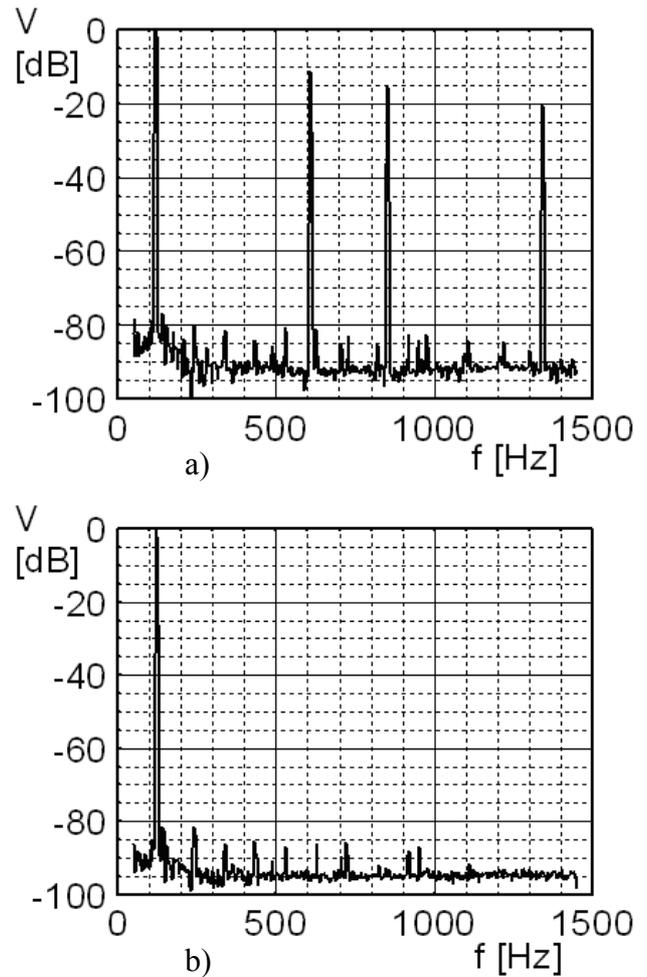
Fig. 3 Frequency spectrum of compound square wave signal a) before filtration b) after filtration
