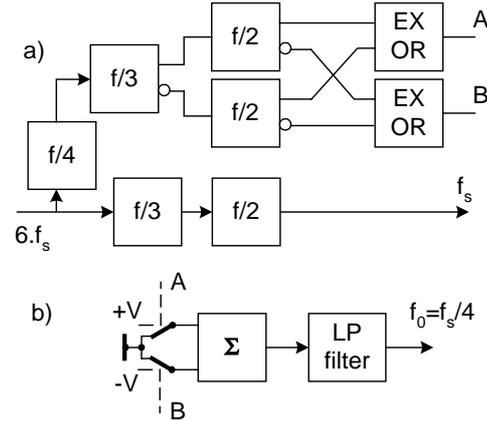
Fig. 2 a) digital part, b) analog part of a generator of the compound square wave signal with rejected 3<sup>rd</sup> harmonic component
