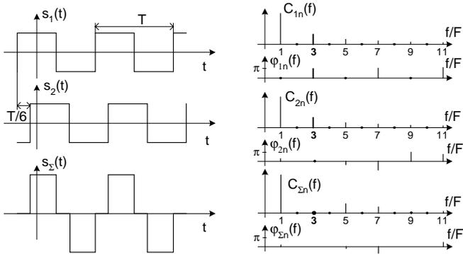
Fig. 1 Square wave signal with zero 3<sup>rd</sup> harmonic component as a sum of two shifted square wave signals.
