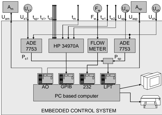
Fig.2 An architecture of the embedded control system
