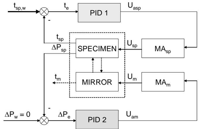
Fig.4 A diagram of the control method with two closed loops
