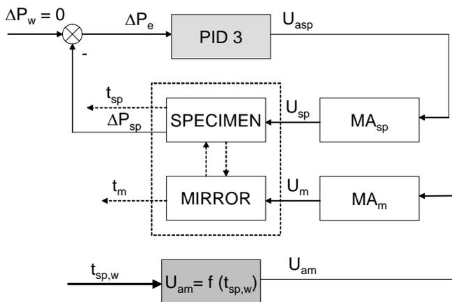
Fig.6 A diagram of the control method with one closed loop
