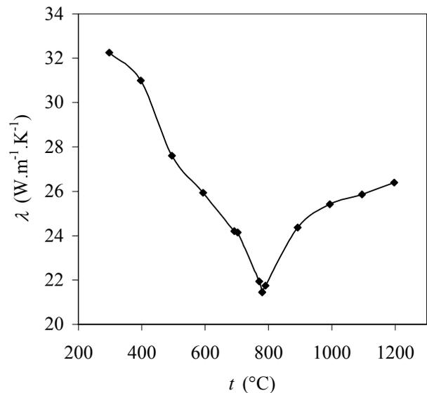
Fig.7 Measured dependence of thermal conductivity coefficient on temperature
