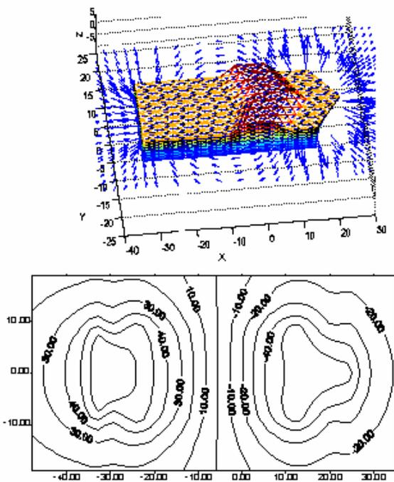
Fig 2-7 lines of magnetic field and magnetic equipotential in the model II Ship type and outside the model.
