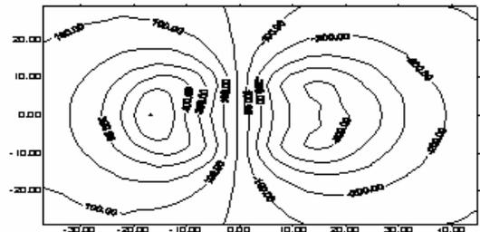
Fig 2-5 lines of magnetic field and magnetic equipotential in the model I Ship type and outside the model.
