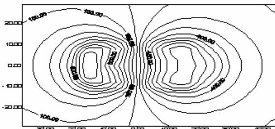
Fig 2-4 lines of magnetic field and magnetic equipotential in the model I Ship type and outside the model.
