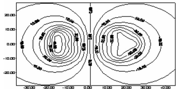
Fig 2-6 lines of magnetic field and magnetic equipotential in the model I Ship type and outside the model.
