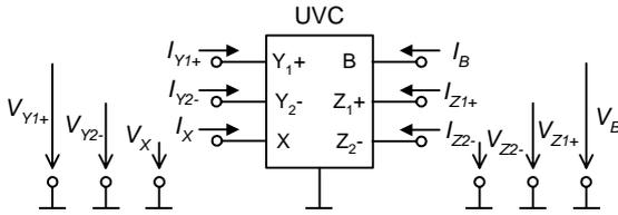
Fig.3 Universal voltage conveyor
