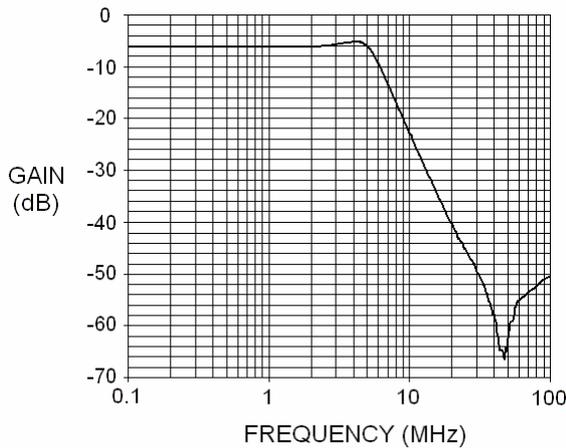
Fig.9 The measured magnitude frequency characteristic of the designed filter
