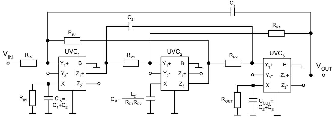
Fig.5 Designed filter with UVCs
