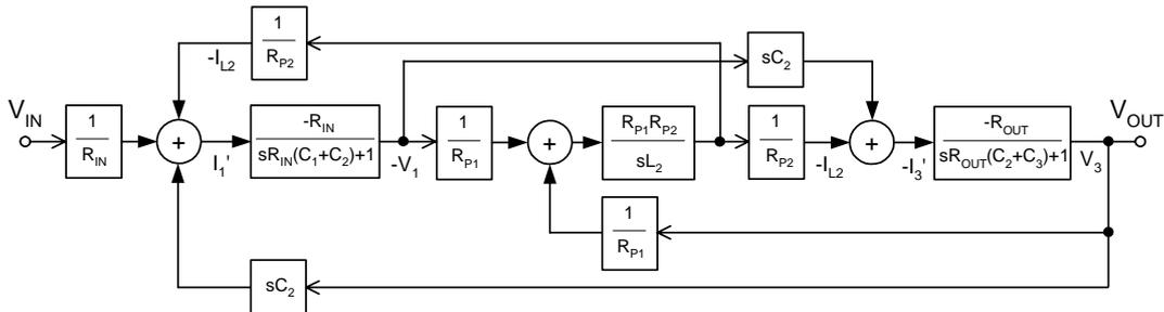
Fig.2 Block diagram derived from RLC filter
