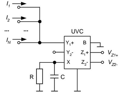
Fig.4 Summing lossy mixed-mode integrator with UVC
