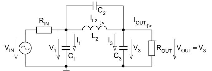
Fig.1. Passive filter prototype chosen for the design
