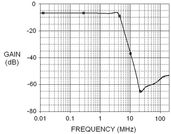
Fig.7 The simulated magnitude frequency characteristic of the designed filter
