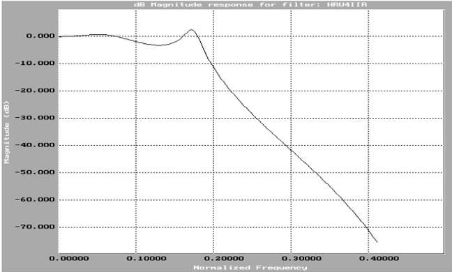
Fig. 6. Frequency response of IIR filter realized by bilinear transformation method.
