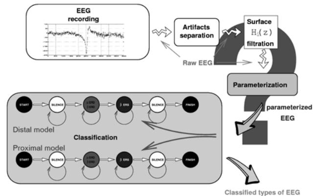
**Fig. 2:** The recorded EEG is analyzed, the epochs with artifacts are discarded. Then the surface filtration follows to increase the SNR of the signal. The signal is parameterized, the appropriate model is selected and the EEG is classified – information is assigned to the realization on the base of the selected distal or proximal models.
