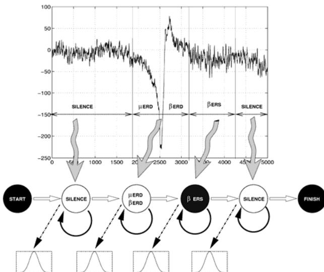
**Fig. 1:** Model architecture and its correspondence to the real EEG shape. The first and last emitting state model the silence before and after the movement. The second emitting state holds the  $\mu/\beta$ ERD characteristics and the third one is related to  $\beta$ ERS.
