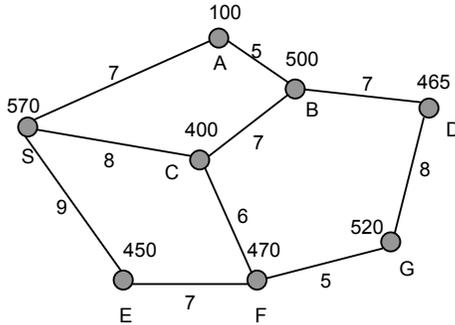
Fig 2: A network with 8 mobile nodes with their battery lifetimes (Network 1).
