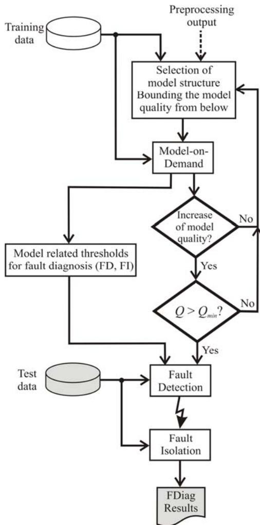
Fig.4. The process of modeling which utilizes the Model-on-Demand, a sophisticated modeling with pre-defined parameters.
