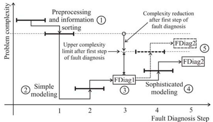
Fig.3. Complexity of a fault diagnosis problem versus steps in fault diagnosis.
