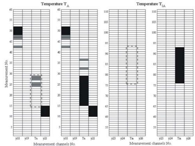
Fig.7. Parts of the fault isolation matrix for the measurement channels  $T_A$  and  $T_{IA}$  after the first level of fault diagnosis (always on left) and after the second level of fault diagnosis (always on right). The black colored boxes indicate likely fault isolations for a specific measurement channel and measurement, while grey colored boxes indicate less likely fault isolations.
