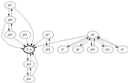
Fig.6. Result of variable selection for measurement channel  $T_A$  as the target channel. The relevance search was done using the stationary data clusters hypothesis.
