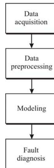
Fig.2. Automatic data plausibility check (fault diagnosis procedure). Basically, the complete fault diagnosis procedure consists of four basic steps: data acquisition, data preprocessing, modeling and fault diagnosis.
