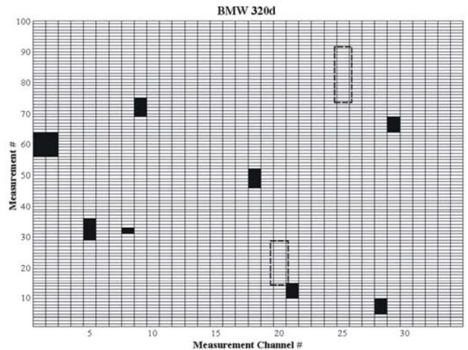
Fig.5. Fault isolation matrix for the BMW 320d data set after the first level of fault diagnosis (using simple modeling).
