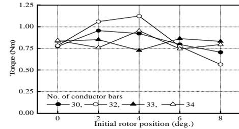
Fig.6 Average torques of the instantaneous starting torques in Fig. 4
