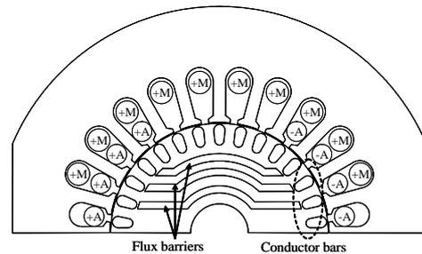
Fig.2 Cross-section of LSsynRM
