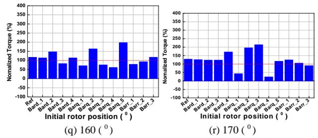
Fig.9 Analysis results of the average starting torque with the initial starting position
