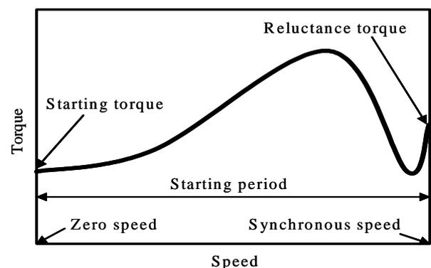
Fig.1 Torque vs. speed of LSsynRM
