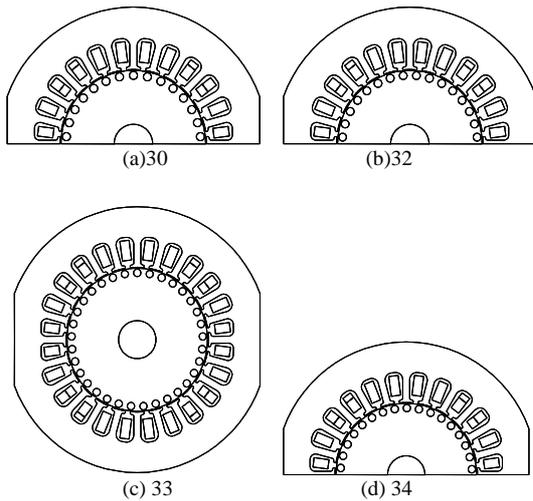
Fig.4 Analysis models with the number of conductor bars
