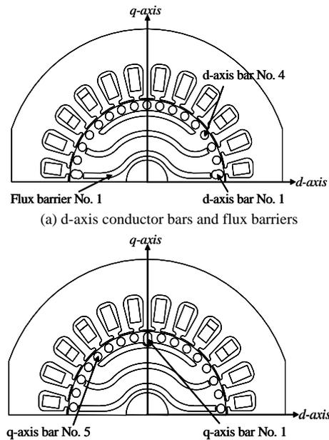
Fig.7 Analysis models with the shape of conductor bars
