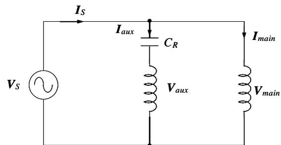
Fig.3 Stator winding connection of LSsynRM
