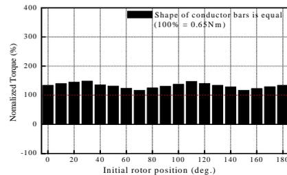
Fig.8 Average starting torques when the analysis models in Fig. 6 are operated as induction motors
