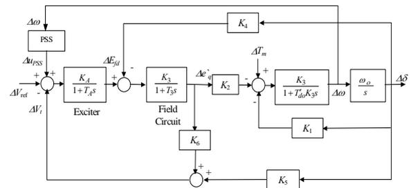
Fig.3: Phillips-Heffron block diagram of SMIBS
