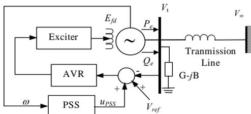
Fig.2: Single Machine Infinite Bus System
