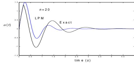
Fig.5-a: Prony fit of the rotor speed,  $n = 20, N = 500$
