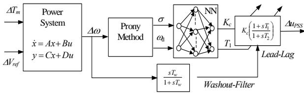
Fig.1: Block schematic of Prony-RBF PSS scheme
