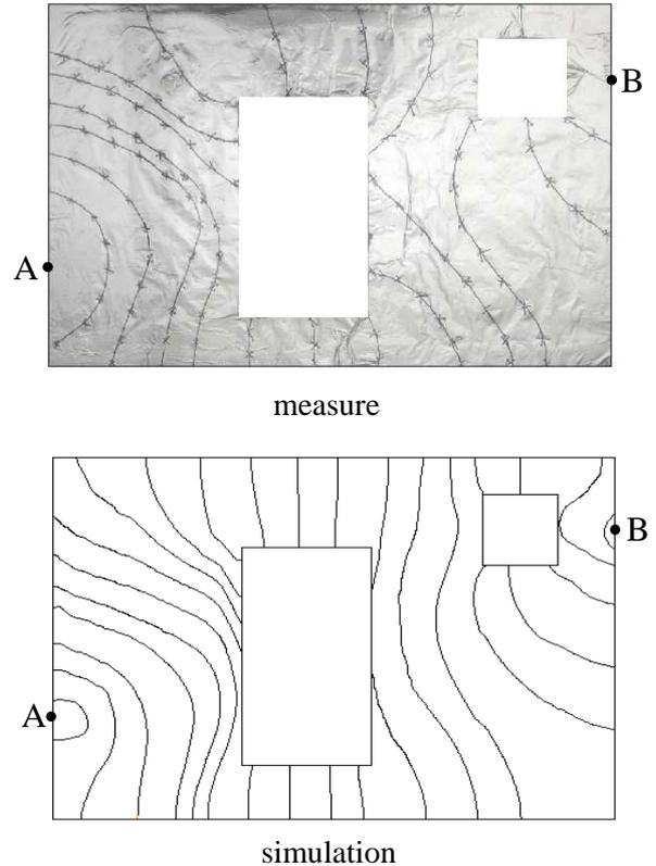
Fig. 5 : simulated equipotential lines using the software IE3D and measured equipotential lines using the probe
