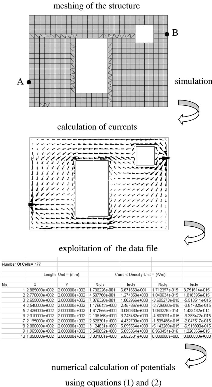
Fig.2 : calculation of potentials from the current simulated by the software IE3D
