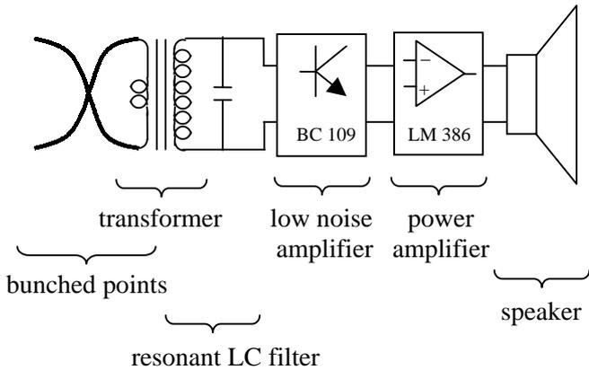
Fig.4 : electronic modules of the probe
