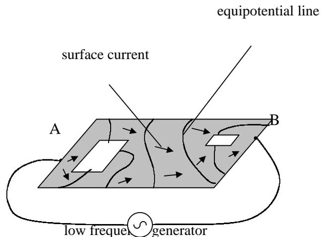
Fig.1 : generation of equipotential lines on a ground plane
