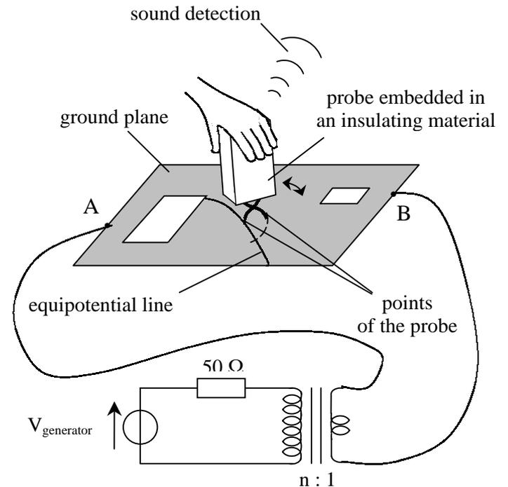
Fig.3 : experimental device to visualize equipotential lines on a ground plane
