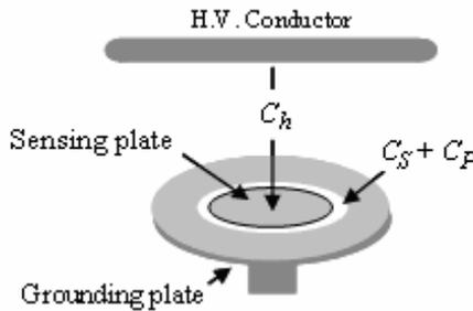
(a) Capacitive Probe Principle
