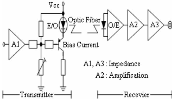
Fig.3 Details of the optical link circuit and assemblies
