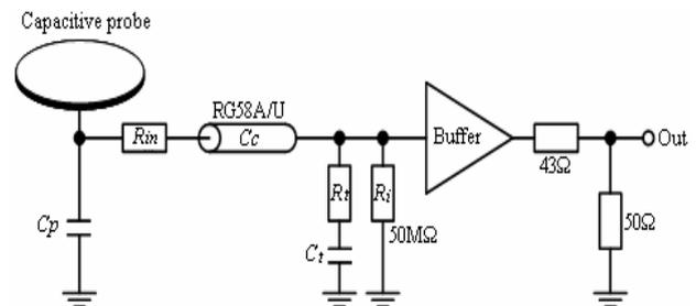
Fig.2 Details of matching of the low voltage arm
