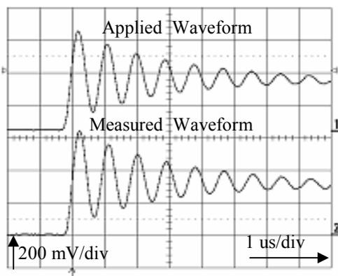
(c) Oscillating impulse voltage
