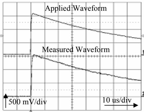
(b) Non-oscillating impulse voltage
