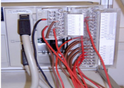
Fig. 10. PLC cards connected using separate conductors (right) and cables with connectors (left)
