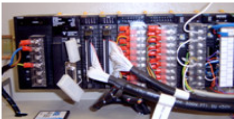
Fig. 13. A modular PLC assembled with cards
