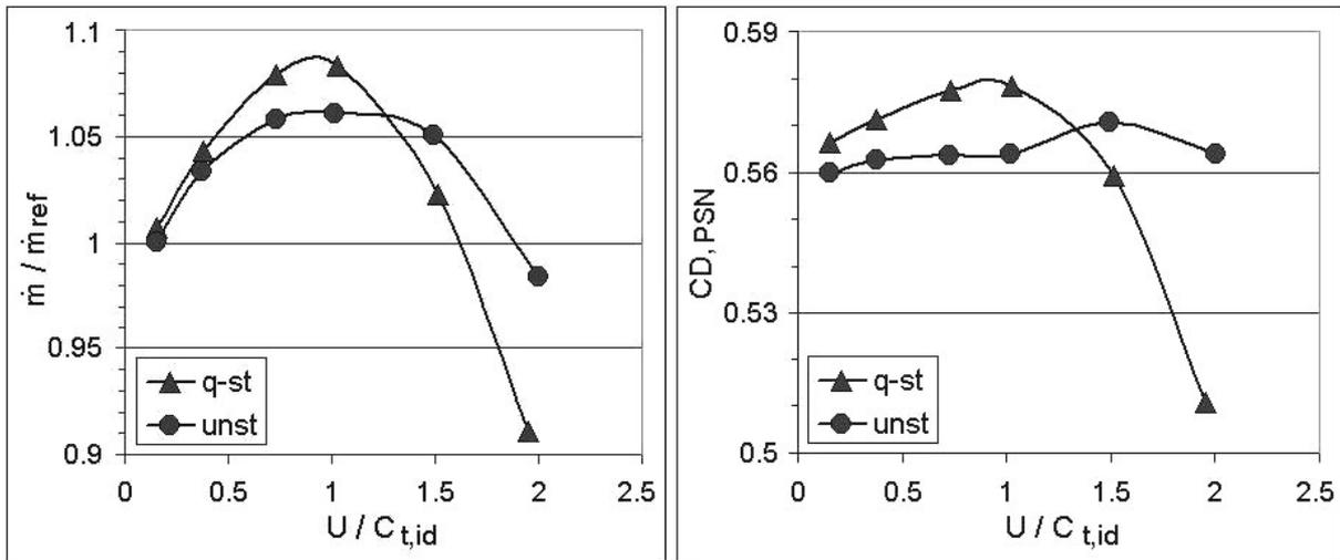
Fig. 6. Mass flow rate (left) and pre-swirl nozzle discharge coefficient (right) as function of velocity ratio  $U/C_{t,id}$ , as predicted by quasi-steady (q-st) and unsteady (unst) approaches.
