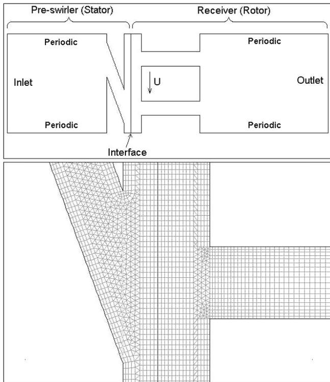
Fig. 1. Solution domain (above) and detail grid (below).
