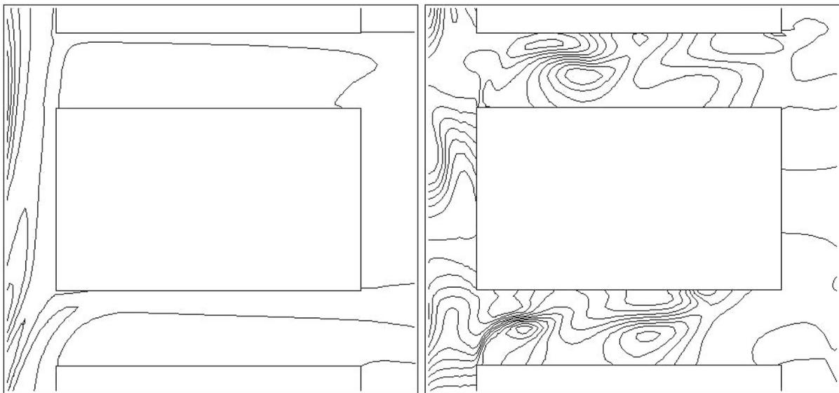
Fig. 4. Predicted isotherms for  $\Pi = 1.2$  and  $U/C_{t,id} = 1.5$ ; Left: Quasi-steady, Right: Unsteady.
