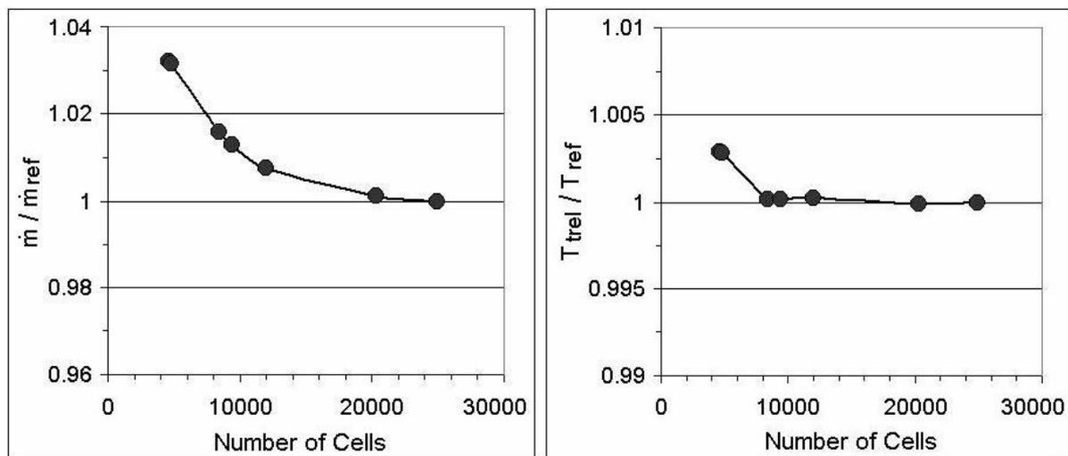
Fig. 2. Variations of mass flow rate (left) and receiver outlet relative total temperature (right) with grid size.
