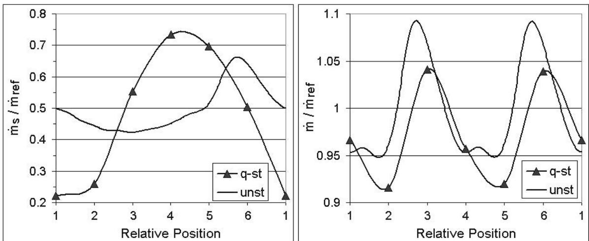
Fig. 5. Variations of mass flow rate with relative stator-rotor positioning for  $\Pi = 1.2$  and  $U/C_{t,id} = 1.5$  as predicted by quasi steady (q-st) and unsteady (unst) approaches; Left: Mass flow rate through a single receiver hole, Right: Total mass flow rate.
