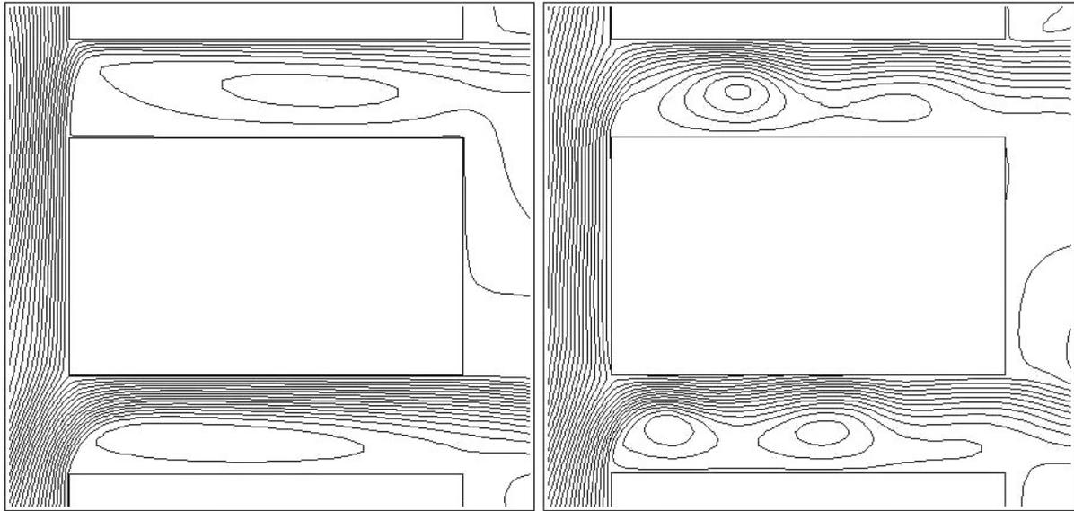
Fig. 3. Predicted streamlines for  $\Pi = 1.2$  and  $U/C_{t,id} = 1.5$ ; Left: Quasi-steady, Right: Unsteady.
