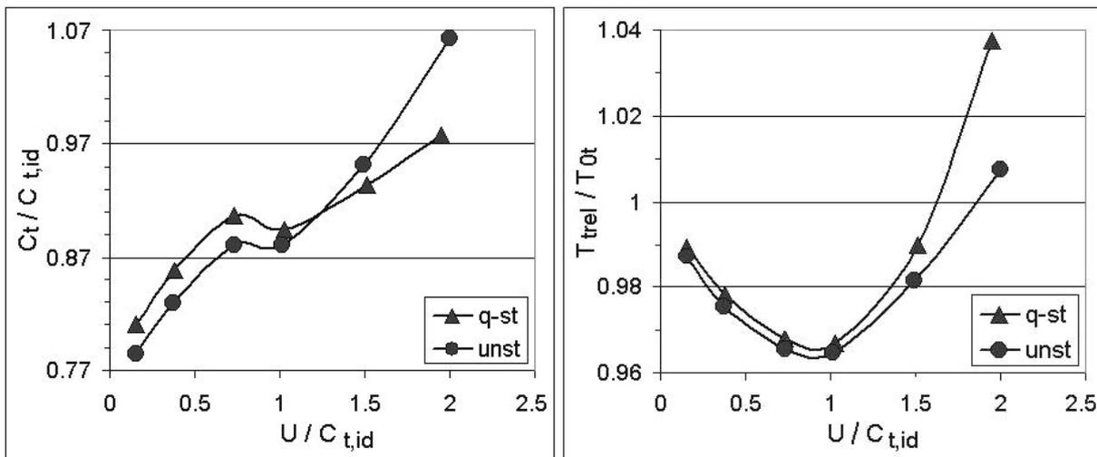
Fig. 7. Non-dimensionalized average tangential velocity at inlet of receiver holes (left) non-dimensionalized average total relative temperature at outlet of receiver holes (right) as function of velocity ratio  $U/C_{t,id}$ , as predicted by quasi-steady (q-st) and unsteady (unst) approaches
