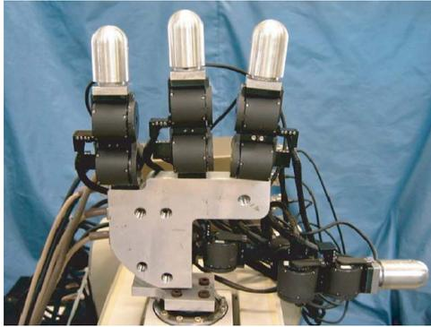
Figure 1: TUT hand with 6-axis force sensor
