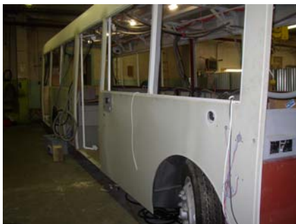
Fig. 6 Assembly of bus with electric drive and monitoring system
