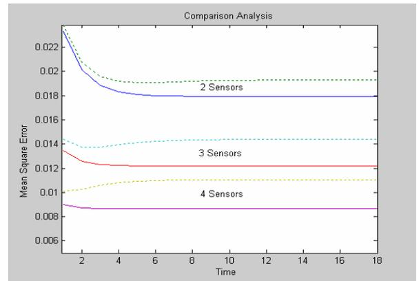
Fig.2. The optimal  $P_k^{\text{opt}}$  (solid line) and suboptimal  $P_k^{\text{sub}}$  (dotted line) mean square errors as a function of number of sensors  $N$ .
