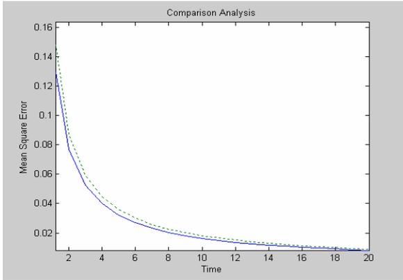
Fig.1. Illustration of the optimal and suboptimal mean square errors:  $P_k^{\text{opt}}$  (solid line) and  $P_k^{\text{sub}}$  (dotted line).
