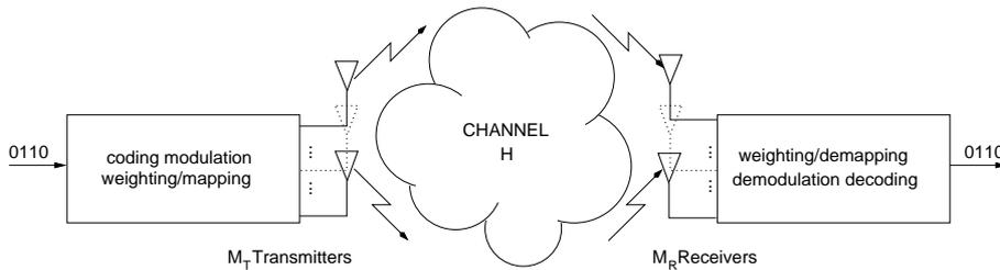
Figure 1: A MIMO system with  $M_T$  transmitting antennas and  $M_R$  receiving antennas.
