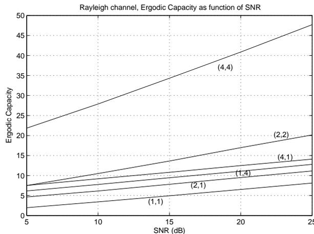
Figure 2: Ergodic capacity for different antenna configurations. The label of each plot line represents the channel  $(M_R \times M_T)$ .
