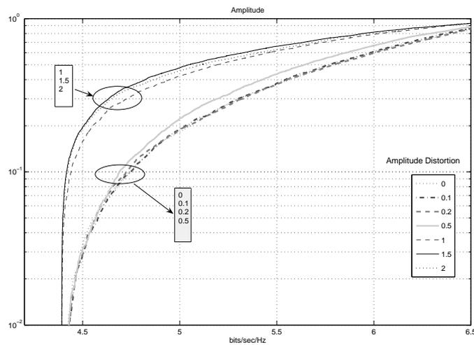
Figure 5: CDF of capacity in the case of a 2x2 channel for different amplitude distortion.
