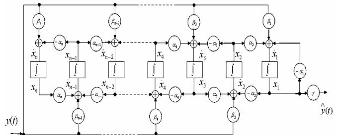
Fig. 4. Internal structure of continuous-time strictly causal system in the dissipation normal form
