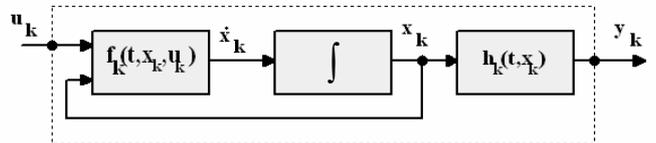
Fig.3. Internal structure of the elementary subsystem  $S_k$
