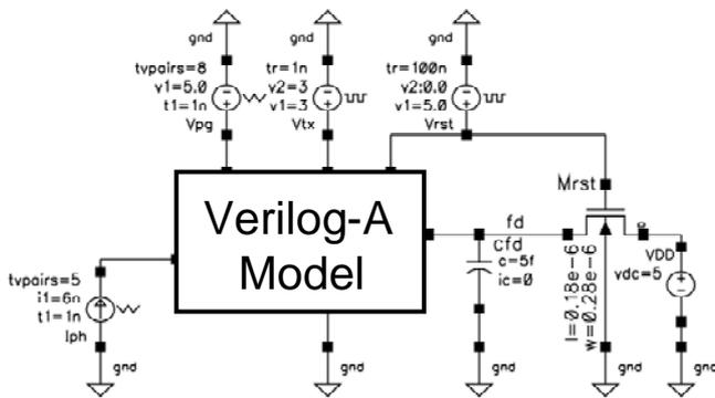
Fig.4: Functional model of a PG APS
