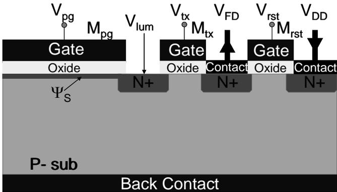
Fig.7: Cut view of a PG and internal potentials
