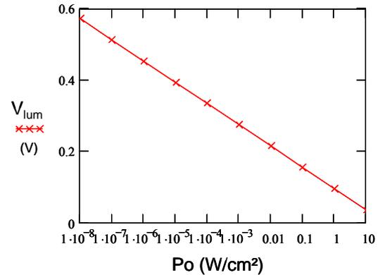
Fig.11: Logarithmic variation of  $V_{lum}$  with  $P_o$
