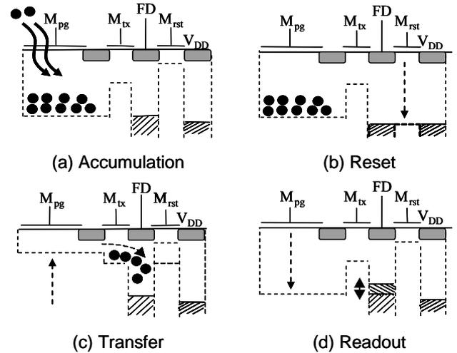
Fig.3: Four steps reading cycle of a PG APS
