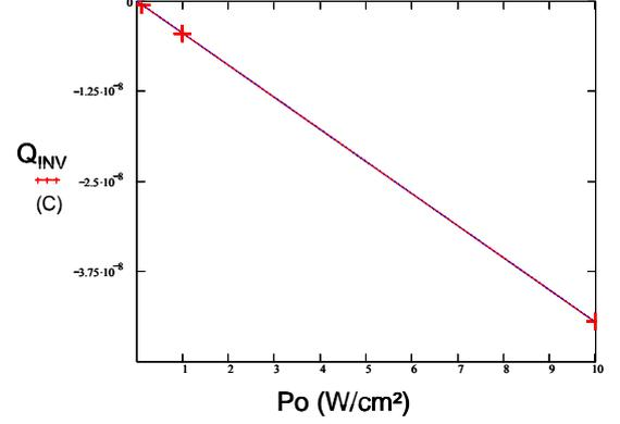
Fig.10: Effect of  $P_o$  light power on  $Q_{INV}$
