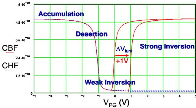
Fig.9: Effect of  $V_{lum}$  on collection capacitance value
