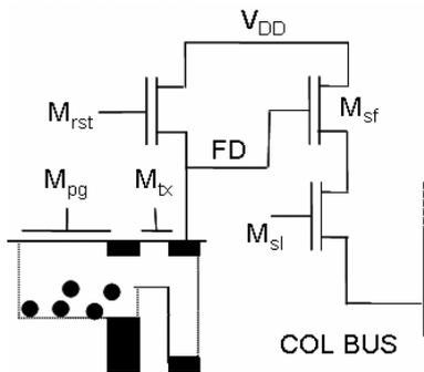
Fig.2: Equivalent schematic of a PG APS
