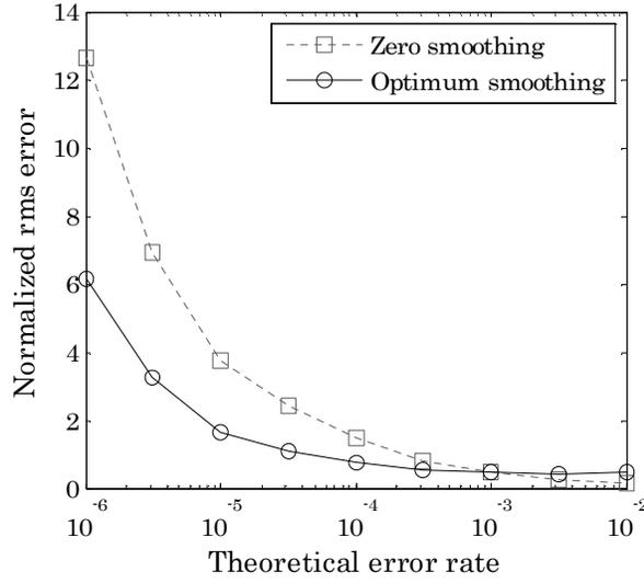
Fig. 1. Normalized rms error of the optimum kernel error monitor and the real-error counting monitor. Each estimate is based on 10000 observations.
