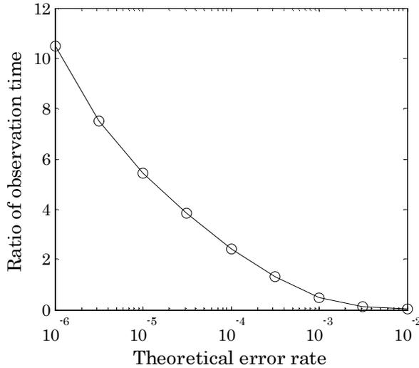
Fig. 2. Ratio of the observation time taken by the real-error counting monitor to that taken by the optimum kernel error monitor to produce ER estimate of equal quality.
