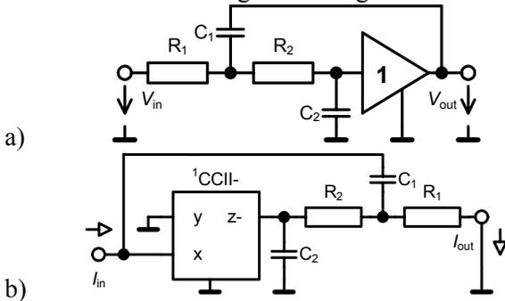
Fig. 3: a) Voltage mode prototype of Sallen Key filter and b) its adjoint counterpart
