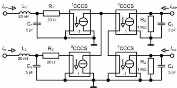
Fig. 14: Model of DCCCS for PSpice environment
