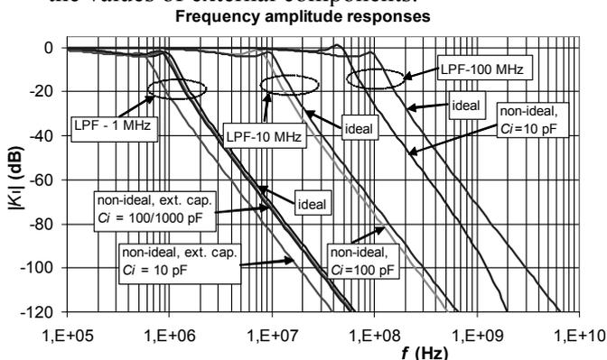
Fig. 15: Frequency responses of the network - Fig. 13
