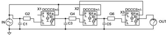
Fig. 13: Third order lowpass filter with DCCCSs
