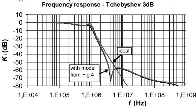
Fig. 8: Frequency responses of the third order Tchebyshev lowpass filter
