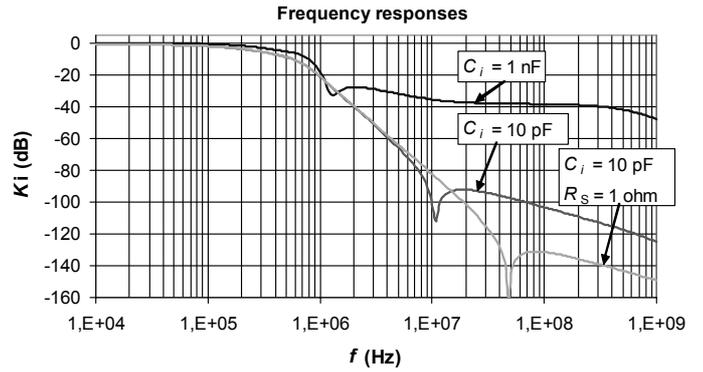
Fig. 10: Influence of the choice of capacitor values in structure from Fig. 7
