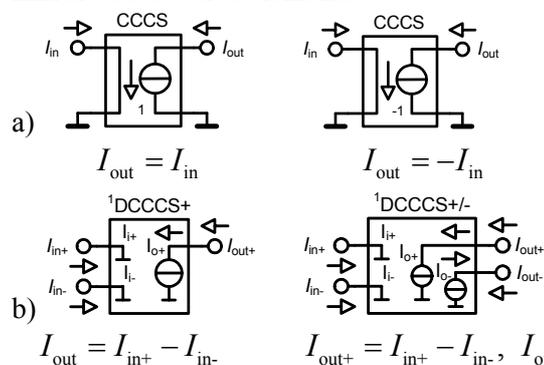
Fig. 1: a) Current mirrors with positive and negative unity transfer, b) differencing current mirrors with single and symmetric current outputs
