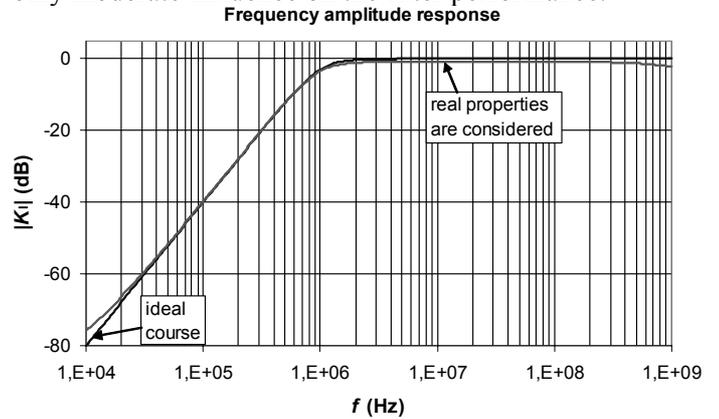
Fig. 6: Frequency response of the second order highpass filter derived from Fig. 3 b)
