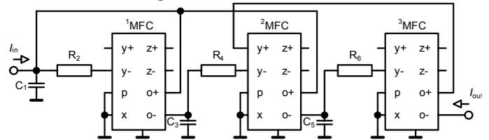
Fig. 16: Realization of the filter from Fig. 13 using MFCs
