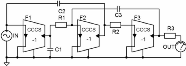
Fig. 7: Third order pure current mode lowpass filter
