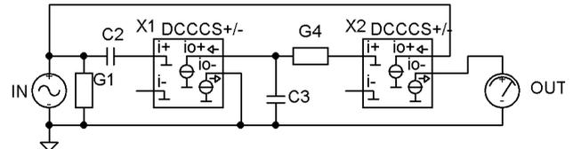
Fig. 12: Second order bandpass filter with DCCCSs
