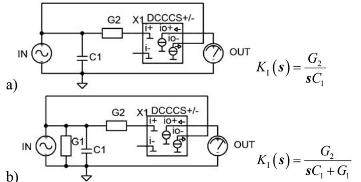
Fig. 11: Lossless and lossy integrators with current mirrors with difference input and symmetrical output
