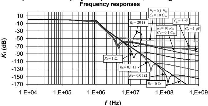
Fig. 9: Frequency responses of the third order lowpass filter under different conditions
