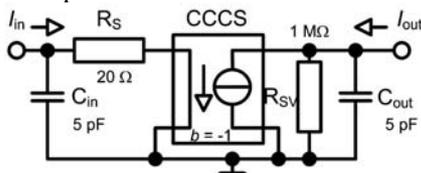
Fig. 4: Model of the current mirror considering some parasitic properties
