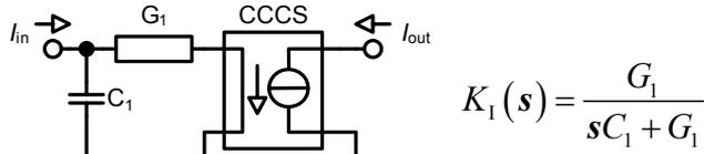
Fig. 2: Current-based lossy integrator
