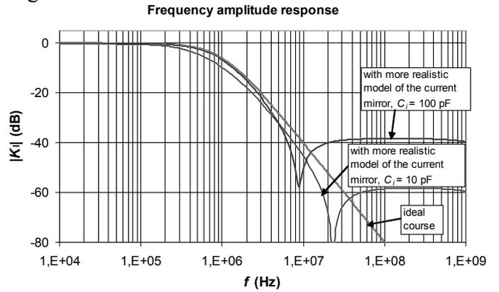
Fig. 5: Frequency responses of the circuit from Fig. 3 b) under different conditions
