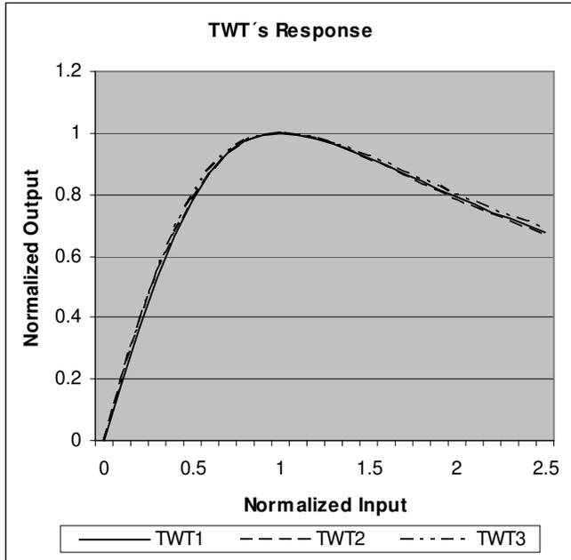
Fig. 3 Normalized TWTA Non-Linear Magnitude Response.
