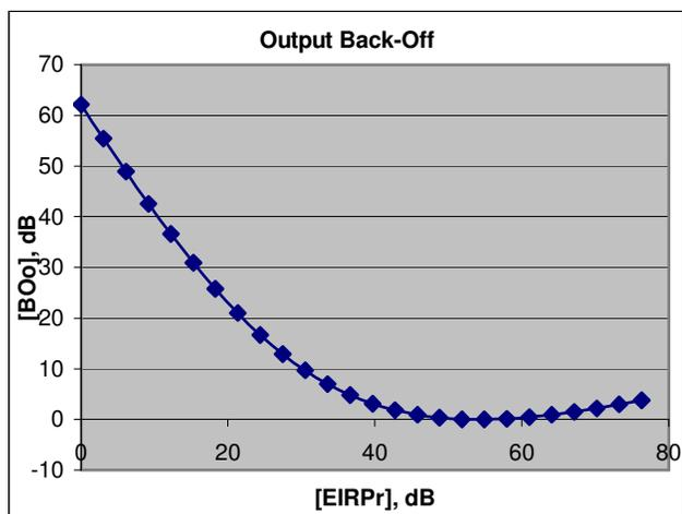
Fig. 4 Output Back-Off using  $TWT_2$
