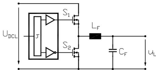
Fig. 1. Conventional switching stage equivalent circuit
