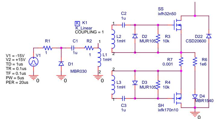
Fig. 5. PSPICE model of the switching stage
