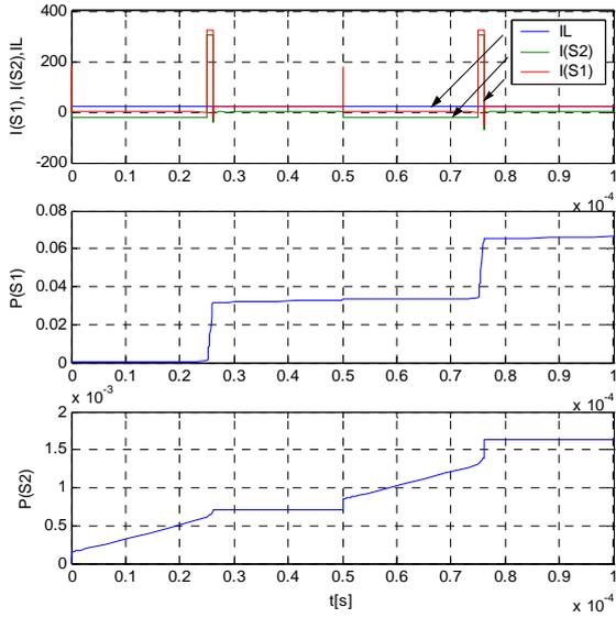
Fig. 6. Half bridge switching leg losses (cf. Fig. 3a):  $S_1$  and  $S_2$  are operated alternatively, unidirectional load current ( $\Delta P_{S1} = 32\text{mWs}$  for test condition)
