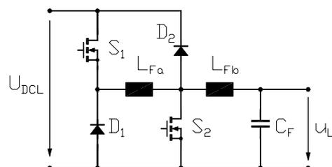
Fig. 2. Improved power switching stages: a.) by path separation, b.) simplified low cost solution
