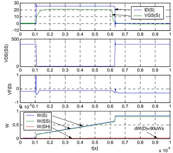
Fig. 8. Switching leg (cf. Fig. 5) with SiC diode SDT12S60 and Schottky clamping diode MBR1530
