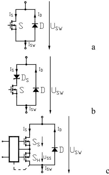
Fig. 3. Improved power switch (derivation):
