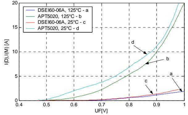
Fig. 4.b Current sharing of MOSFET APT5020 & Diode DSEI60-06A (cf. Fig. 3.a):
