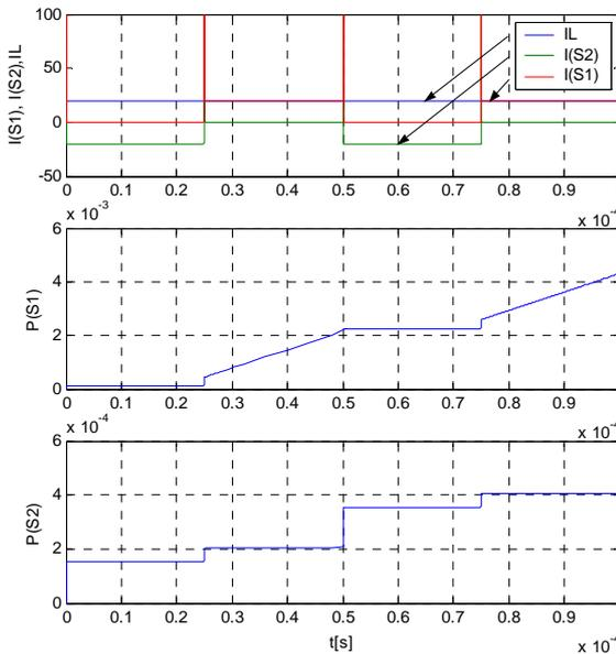
Fig. 7. Half bridge switching leg losses (cf. Fig. 3b)  $S_1$  and  $S_2$  operated alternatively, unidirectional load current ( $\Delta P_{SS} = 0.35\text{mWs}$  for test condition)
