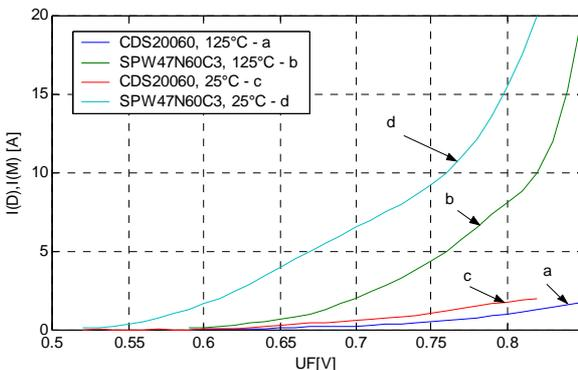
Fig. 4.a Current sharing of MOSFET SPW47N60C3 & Diode CSD20060 (cf. Fig. 3a).
