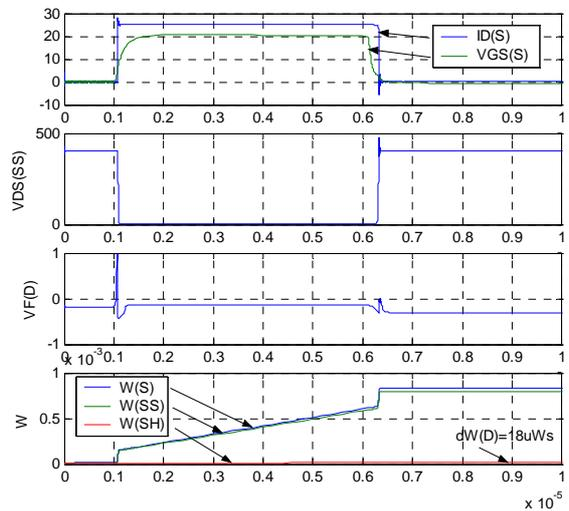
Fig. 9. Switching leg (cf. Fig. 5) with SiC diode SDT12S60 and active (MOSFET) clamping
