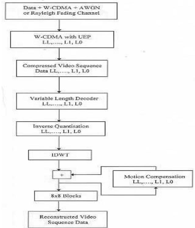
Fig. 2 Block Diagram of Multilevel UEP Codes for Wavelet Video Transmission in W-CDMA system over AWGN and Rayleigh fading channels Decoder
