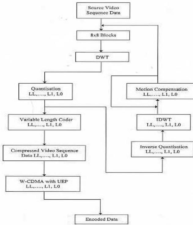
Fig. 1 Block Diagram of Multilevel UEP Codes for Wavelet Video Transmission in W-CDMA system over AWGN and Rayleigh fading channels Encoder
