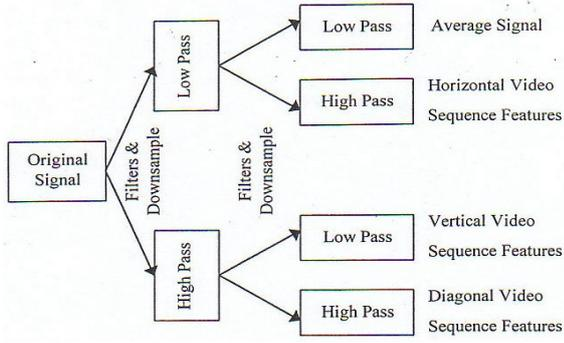
Fig. 4 Wavelet Decomposition of the 2-D Wavelet Packet Transform for the Video sequence
