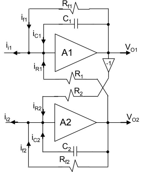
Figure 3. Simple active polyphase filter for analysis
