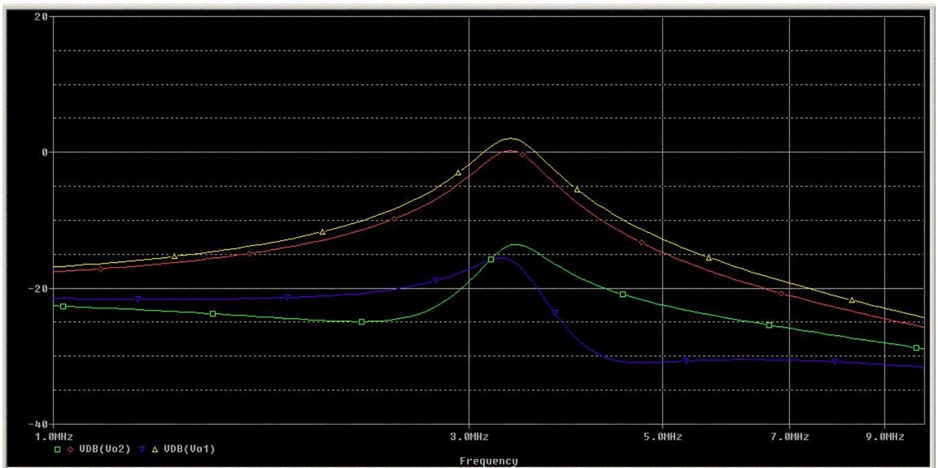
Fig. 4 The gain-frequency characteristics of the polyphase filter realization of Fig. 2
