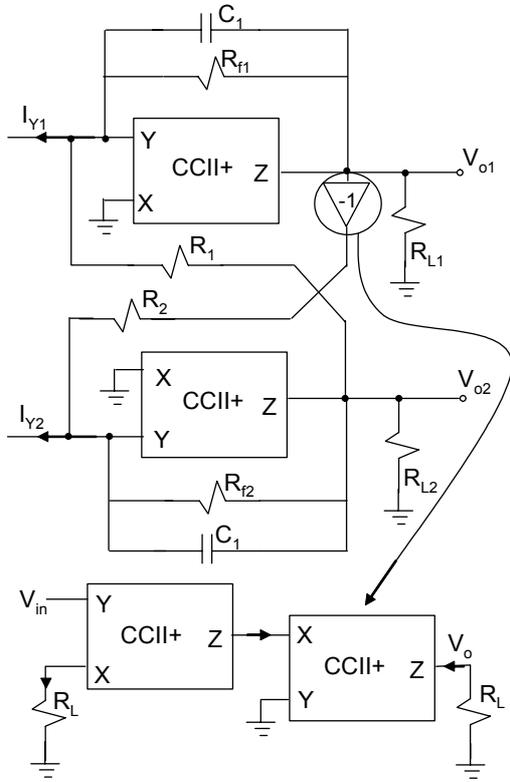
Figure 2. The proposed active polyphase filter using CCII+
