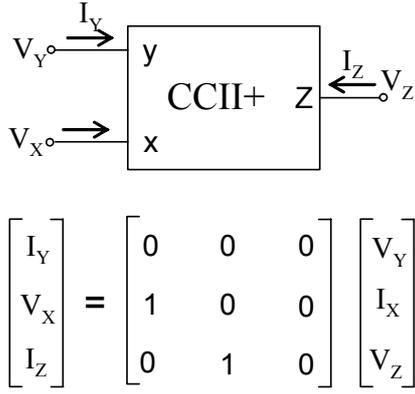
Figure 1. Symbol representation of CCII+ and its transfer function
