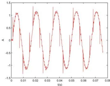
Fig. 7 – Compensated currents with Kalman filtering and AFPLL
