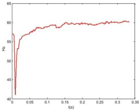
Fig. 2 – Identification of frequency with RLS
