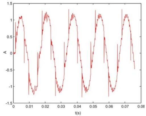
Fig. 4 – Compensated currents with Kalman filtering and RLS
