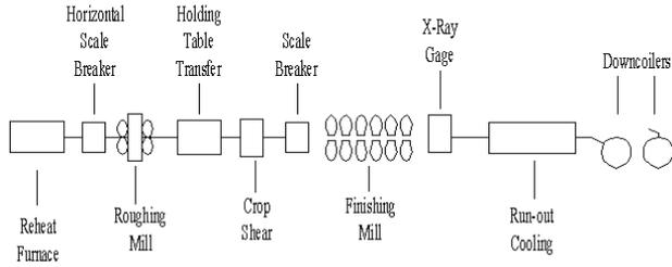
Fig. 1 Typical Hot Strip Mill (HSM)
