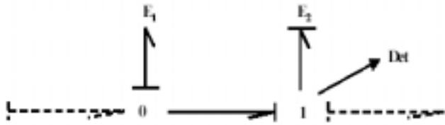
Fig. 7 Case of two different junctions representing the combination  $[0\ 1]$
