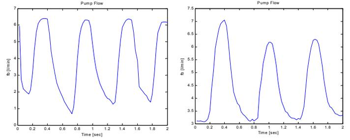
Fig. 2.  $P_{ao}(t)$ ,  $P_{Vi}(t)$  and  $f_b(t)$  recorded from the ex-vivo tests, corresponding to  $n_1 = 7200$  rpm (left side) and  $n_1 = 8100$  rpm (right side).
