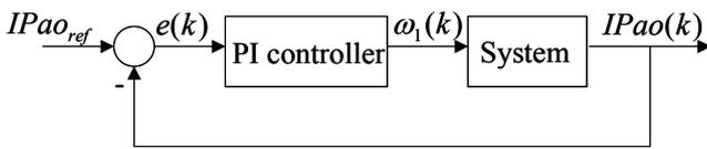
Fig. 8 Block diagram for calculation  $k_p$  and  $k_i$ .
