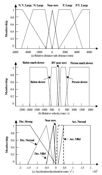
Fig. 3 Membership functions for the fuzzy system input and output variables.
