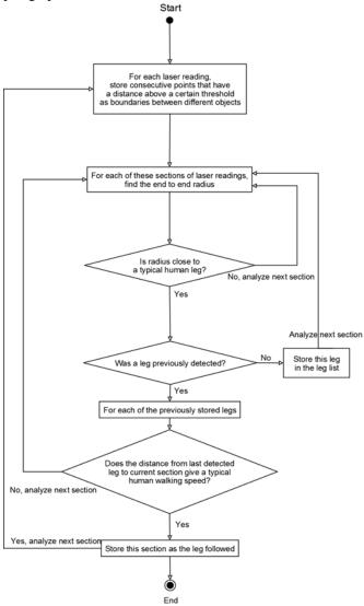
Fig. 1 Leg Detection Algorithm
