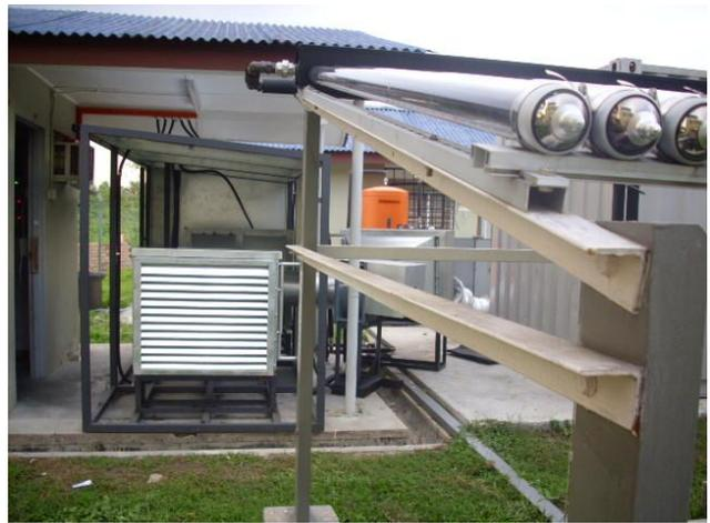
Fig.3 the solar desiccant drying system
