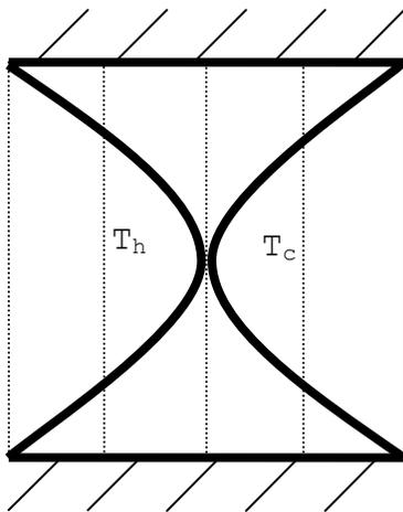
Figure 1d Severely scalloped module with  $\frac{\delta_{\min}}{L} \approx 0$
