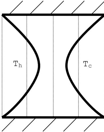
Figure 1c Moderately scalloped module with  $\frac{\delta_{\min}}{L} = 1/4$
