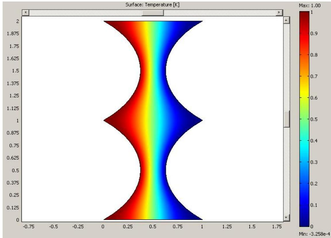
Figure 2c Isotherms plot for the moderately scalloped module with  $\frac{\delta_{\min}}{L} = 1/4$
