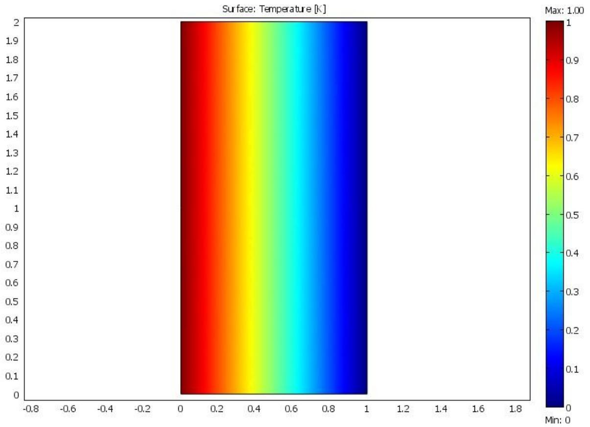
Figure 2a Isotherms plot for the square module
