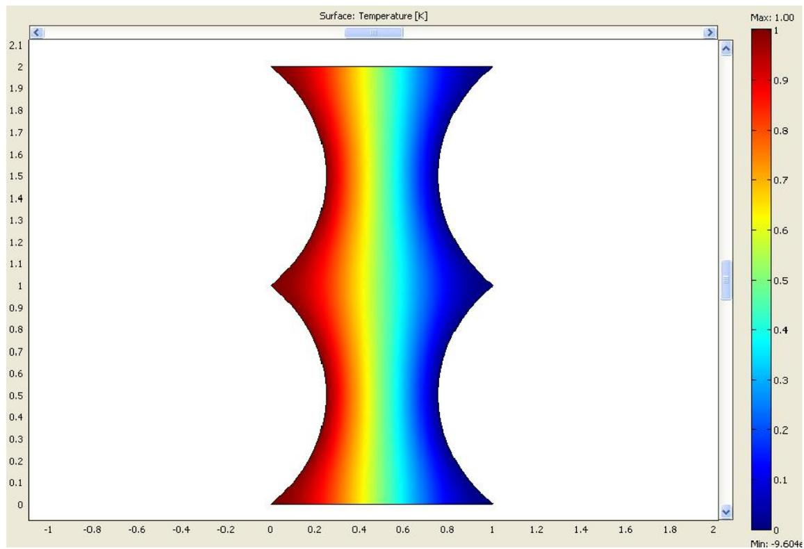
Figure 2b Isotherms plot for the slightly scalloped module with  $\frac{\delta_{\min}}{L} = 1/2$
