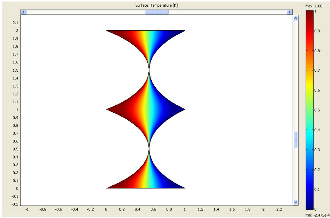
Figure 2d Isotherms plot for the severely scalloped module with  $\frac{\delta_{\min}}{L} \approx 0$
