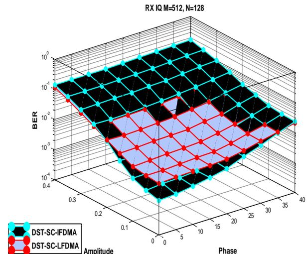
**Fig.5:** BER against Amplitude and Phase of DST-SC-IFDMA and DST-SC-LFDMA systems with RX IQI scenario.
