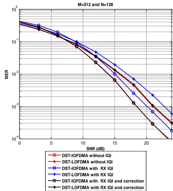
**Fig.9:** BER against SNR for DST-OFDMA system with RX IQI correction scheme
