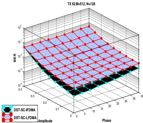
**Fig.3:** BER against amplitude and Phase of DST-SC-IFDMA and DST-SC-LFDMA systems with TX IQI scenario.
