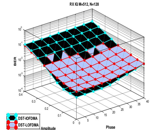
**Fig.6:** BER against Amplitude and Phase of DST-IOFDMA and DST-LOFDMA systems with RX IQI scenario.
