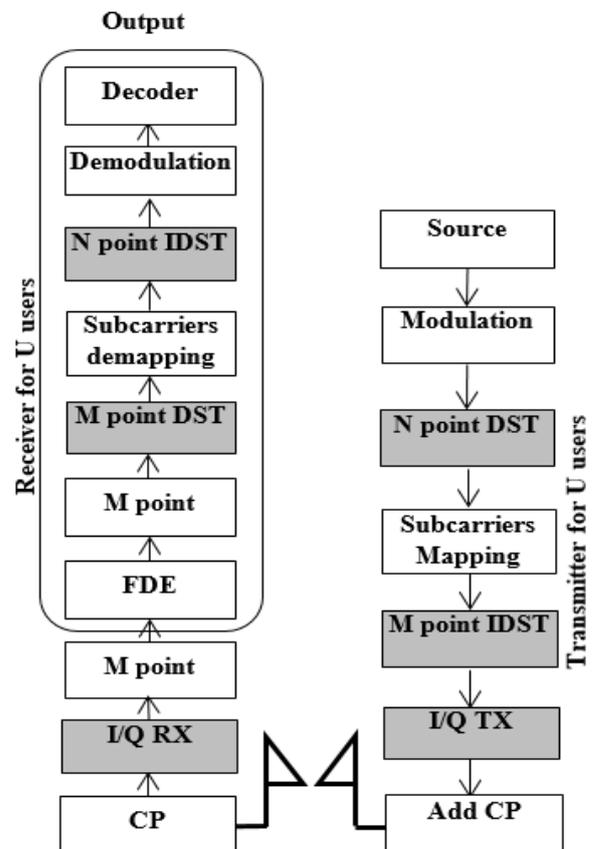
**Fig.2:** Transceiver structure of the DST-SC-FDMA system with TX-RX IQI scenario
