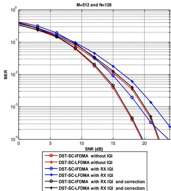
**Fig.10:** BER against SNR for DST-SC-FDMA system with RX IQI correction scheme
