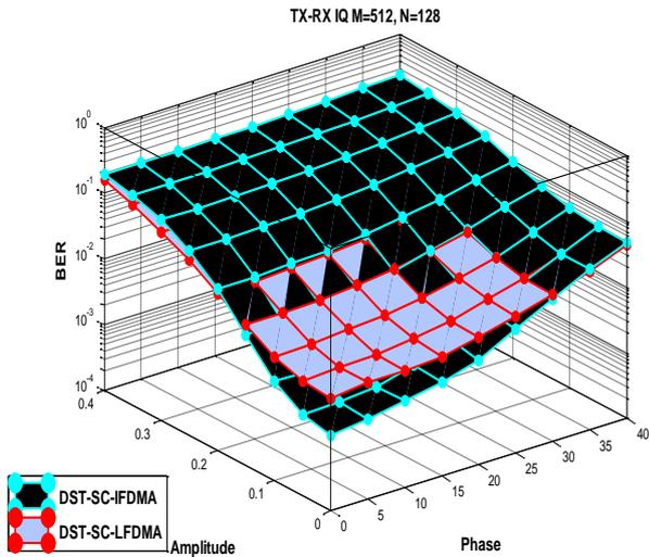
**Fig.7:** BER against Amplitude and Phase of DST-SC-IFDMA and the DST-SC-LFDMA systems with TX-RX IQI scenario.
