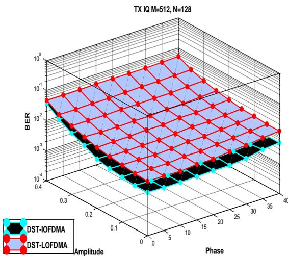
**Fig.4:** BER against Amplitude and Phase of DST-IOFDMA and DST-LOFDMA systems with TX IQI scenario.
