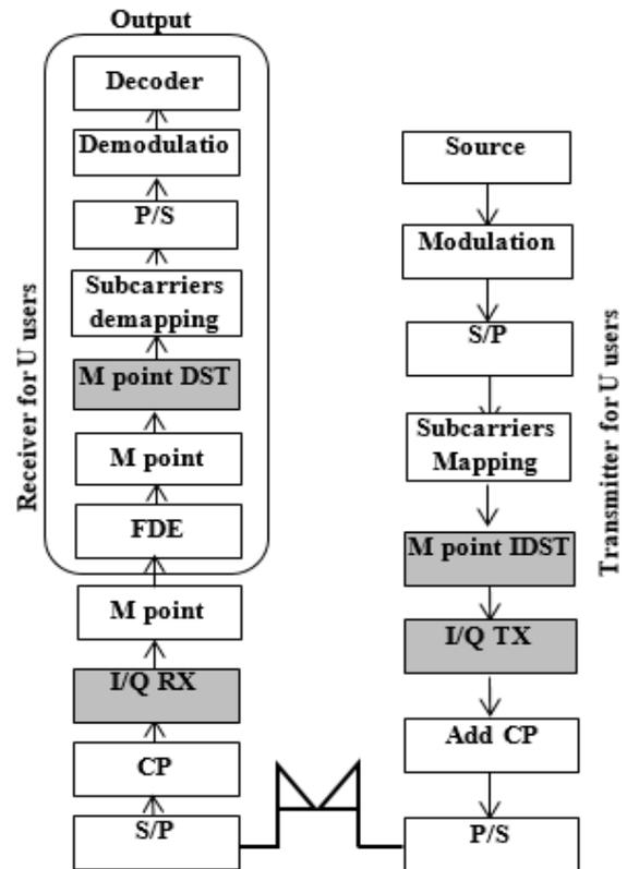
**Fig.1:** Transceiver structure of the DST-OFDMA system with TX-RX IQI scenario
