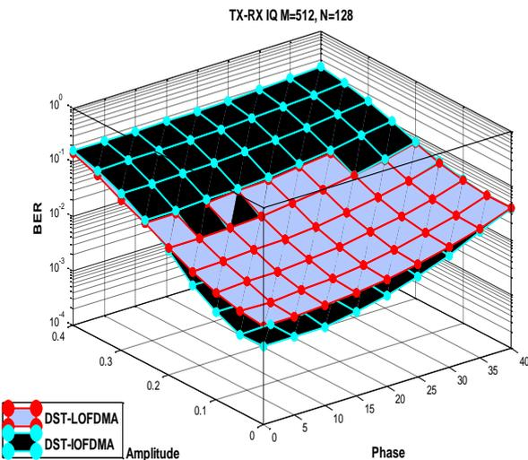
**Fig.8:** BER against Amplitude and Phase of DST-IOFDMA and the DST-LOFDMA systems with TX-RX IQI scenario
