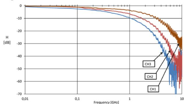
Fig.1 Transfer functions of real transmission channels
