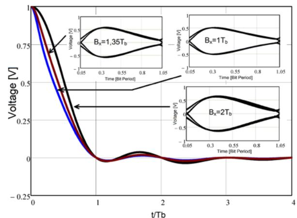
Fig.9 Impulse response and eye diagram performance for various  $T_b$ .
