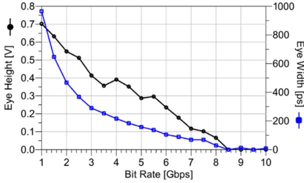
Fig.3 Output eye diagram analysis, conventional pulse
