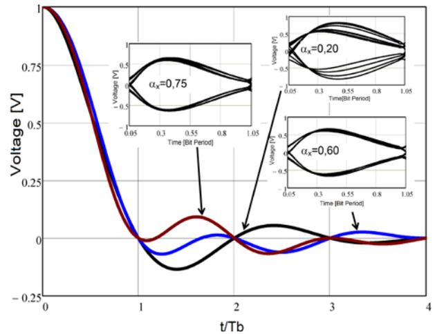
Fig.8 Impulse response and eye diagram performance for various  $\alpha_x$ .
