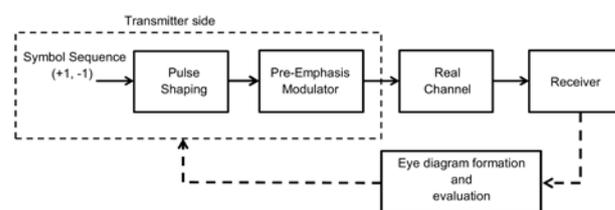
Fig.2 Simple schematic of proposed/modeled communication chain
