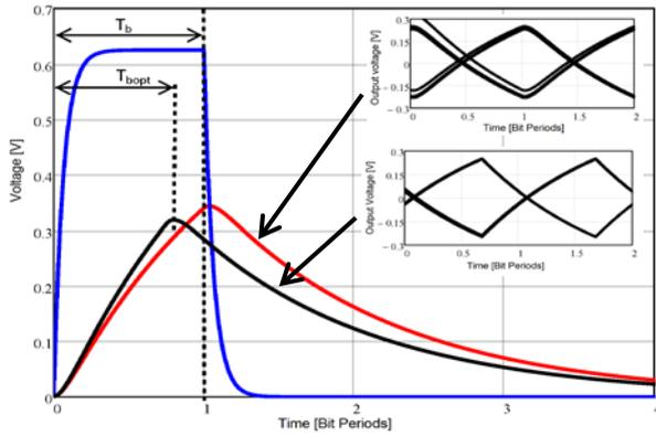
Fig.5 Output eye diagram analysis, optimized pulse
