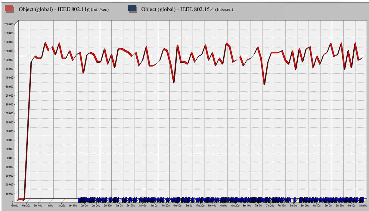
Fig. 7. Global statistics – Throughput (bits/sec) comparison for both protocols
