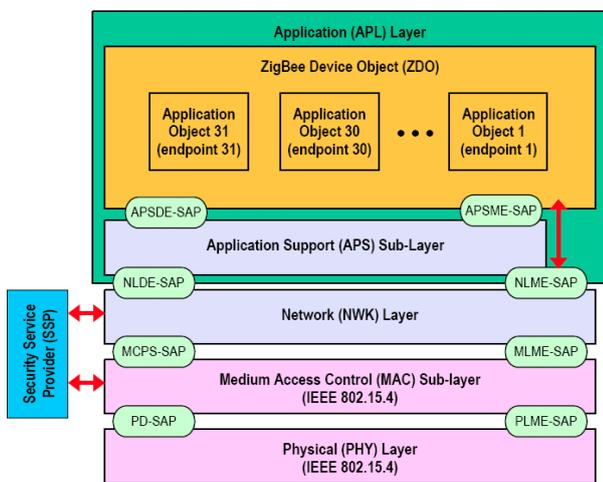
Fig. 1 ZigBee Communication Stack
