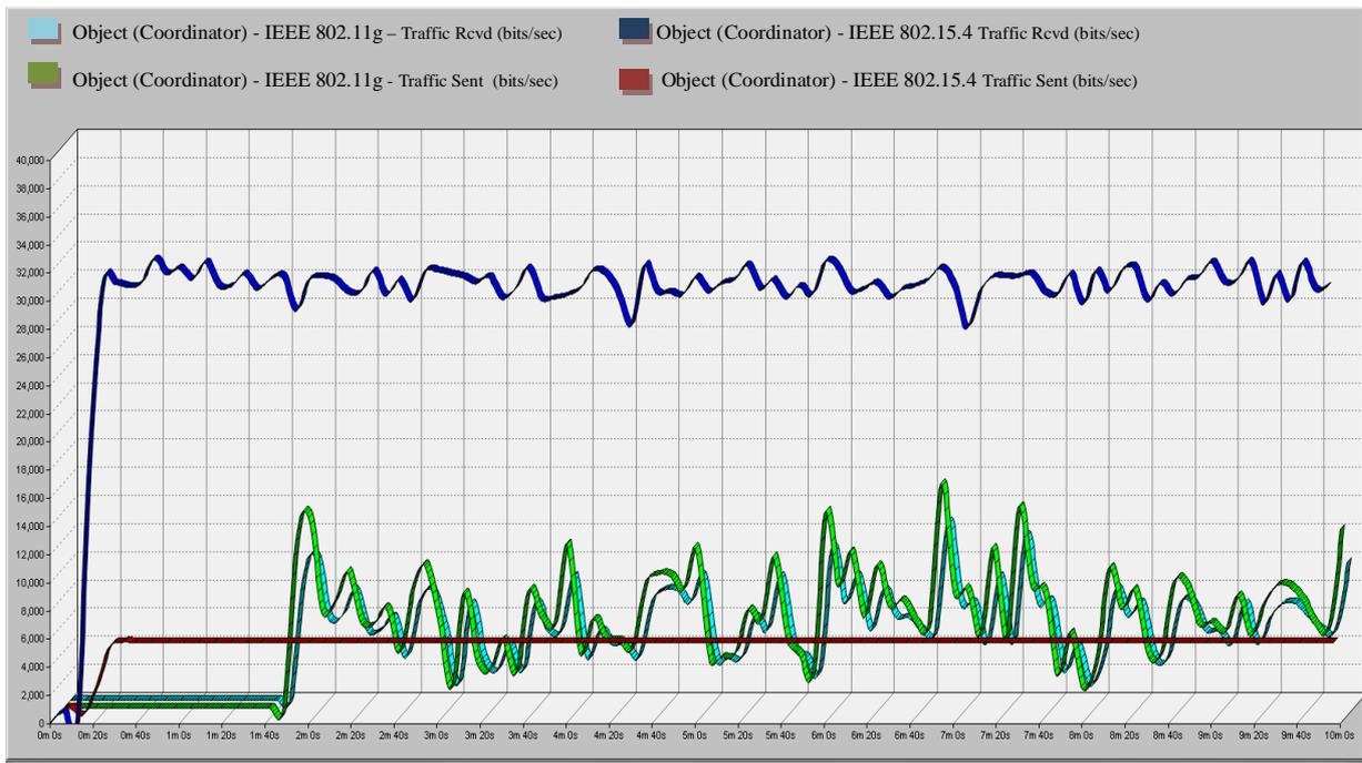
Fig. 9. Coordinator statistics -Traffic received, Traffic sent (bits/sec) comparison for both protocols
