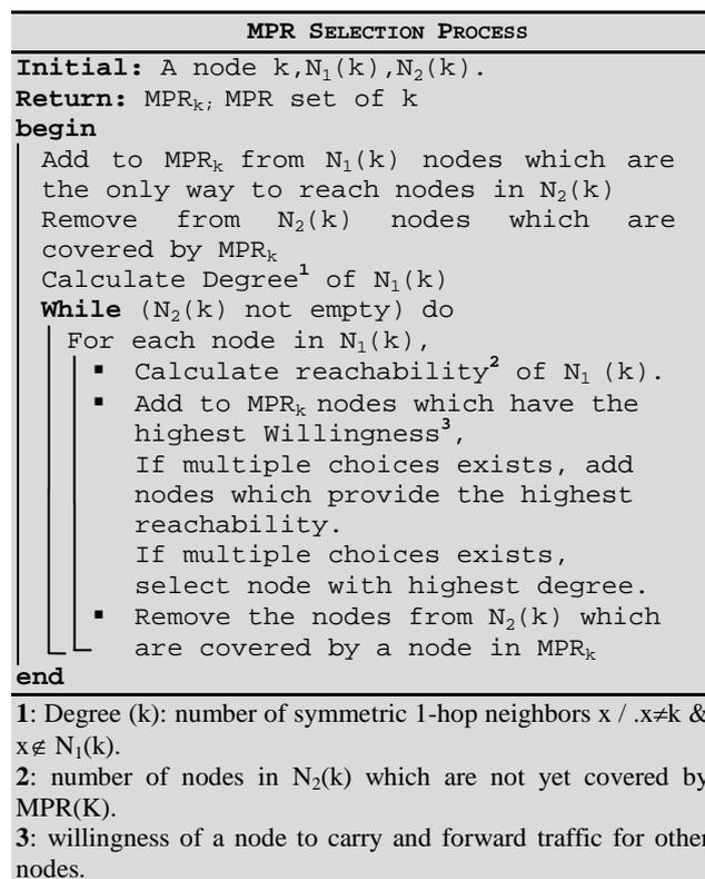
Fig.1 MPR-set construction algorithm
