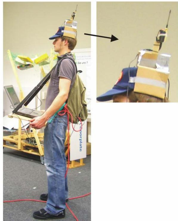
Figure 9. Mobile sensor node on top of user's head
