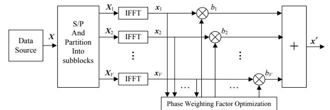
Figure 1: Block diagram of CPTS scheme
