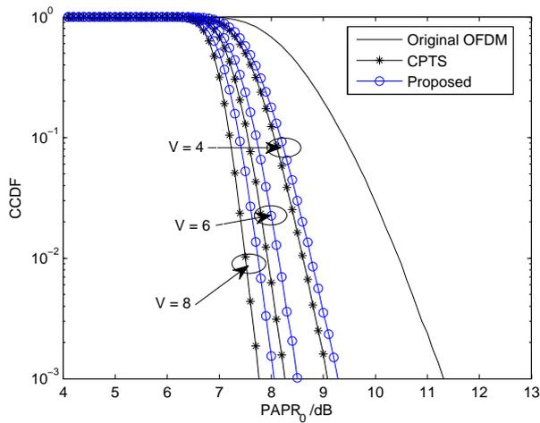
Figure 2: Comparisons in PAPR reduction performance between proposed PTS and CPTS when the number of subblocks is even
