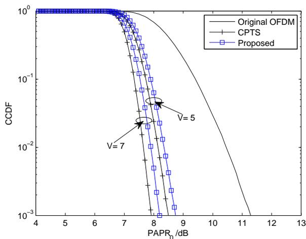
Figure 3: Comparisons in PAPR reduction performance between proposed PTS and CPTS when the number of subblocks is odd
