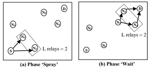
Fig.3: Spray and Wait Routing.
