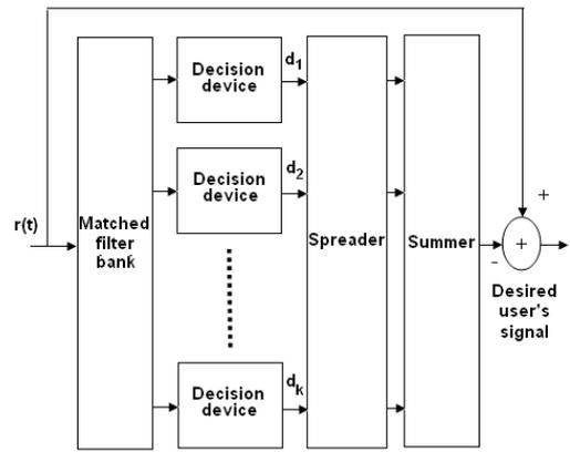
Fig.4. Block diagram of Parallel interference cancellation receiver
