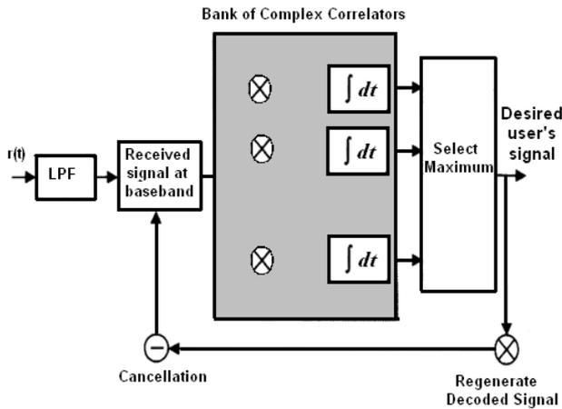
Fig.3. Block diagram of successive interference cancellation receiver
