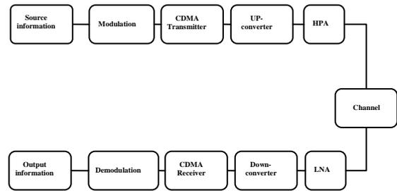
Fig 7. Overall Simulation Block Diagram
