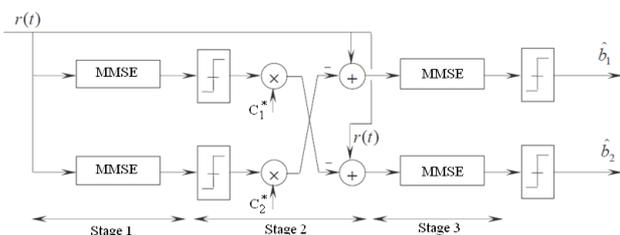
Fig.6. Block diagram of combined detection (MMSE/PIC)
